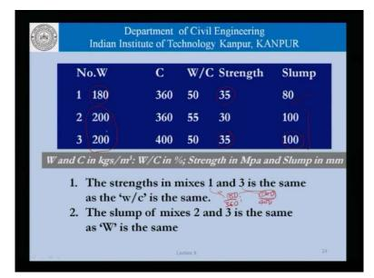
It means in numerical terms as an example is shown here, if we have three mixes 1,2 and 3 and they have water content these values are in k g per cubic meter and water cement ratio is in percentage the strength is in m p a and the slump is in millimeter. Now, if 180,
