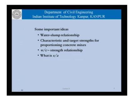
We have gone through some of these very important ideas which govern our proportioning exercise. This is the water slump relationship the characteristics and target strength for proportioning concrete mixes water cement ratio versus strength relationship and the importance of s by a.
