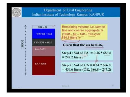
This means that the remaining volume that is sum of the fine and the coarse aggregate which is a 1,000 liters that is what is the total volume this is the volume of the air volume of water volume of cement. The total volume for inert material left to us is 686.8 liters and this has to be proportion in the fine aggregate and coarse aggregate given that the s by a is 0.36, the volume of the fine aggregate is 0.36 multiplied by this volume that we have for all the inert material.
