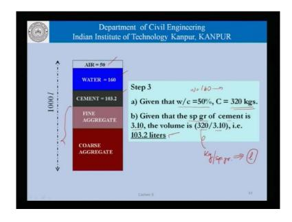
That was in the previous slide and with this information we are now going to embark upon the process of determining the relative volumes of air water cement fine aggregate and coarse aggregate as we have been doing. Now, the first thing that is given to us is that that is 50 liters of air given that the air content is 5 percent by volume 1,000 liters of the volume of the pitcher.
