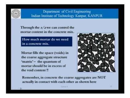
In other words, s by a is used to control the amount of mortar in the concrete mix and how much do we need. How much of mortar, do we need in the concrete mix is determined by the type of coarse aggregate the size of the coarse aggregate, its properties particle size distribution and so on.
