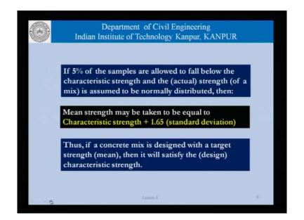
The concrete proportioning has to be carried out using what was called the target proportioning strength of concrete. The target strength of concrete which is basically the strength of the mix that we used and that has to be determined in a manner that the characteristic strength criteria is satisfied.
