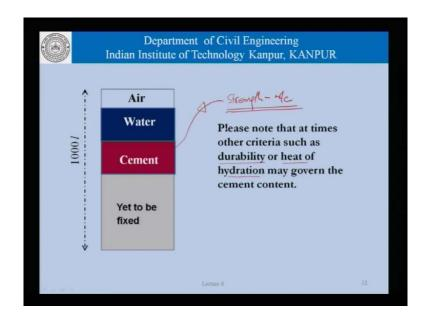
So, going back to that model where we are trying to proportion the thousand liters which is the absolute volume of the pitcher we already knew the air content we knew the water content from the slump water content relationship. We now know the cement content from the water cement ratio relationship with strength the remaining part is still to be fixed.
