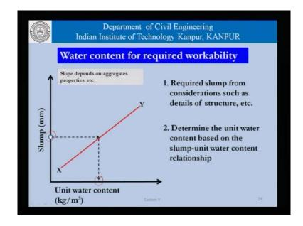
Now, we come to the unit water content in slump requirement, we told we have to know the required slump what is the slump that we need for the particular concrete depending on parameter such as the details of the structure. If the structure for example, has a lot of dense reinforcement we may need that the concrete should have higher slump. If the concrete has to be placed in a structure, which has very nominal amount of reinforcement we may be able to make do with a slump which is very small.
