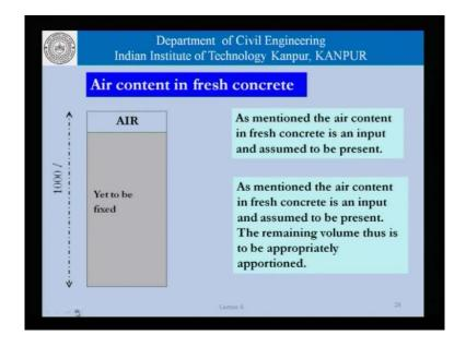
As far as the air content in fresh concrete is concerned that is the first step, so given that we are trying to work with a 1,000 liters that is the pitcher volume the air content in fresh concrete is an input. It is assumed to be known for the present and what we are left with this to fix the remaining volume in the 1,000 liters.
