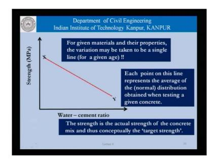
Carrying on, from our previous discussion we had said that much like the relationship between slump and unit content the relationship between strength. The water cement ratio can be taken to be a simple straight line in a manner that as the water cement ratio increases the strength decreases. Each point on the line really represents the mean of the normal distribution of strength that we get when we test a large number of concrete cubes or concrete samples at a given water cement ratio.
