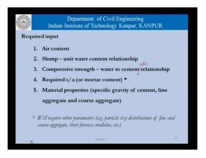
We have durability requirements or any other requirements that may be imposed on the concrete mix in terms of water cement ratio which can be said that it should not exceed 50 percent or 45 percent. Similarly, that can be restriction on the use of cement to be at least 400 kgs per cubic meter or at most 350 kg s per cubic meter and so on. So, with these governing considerations, we proceed to carry out the portioning of concrete mixes
