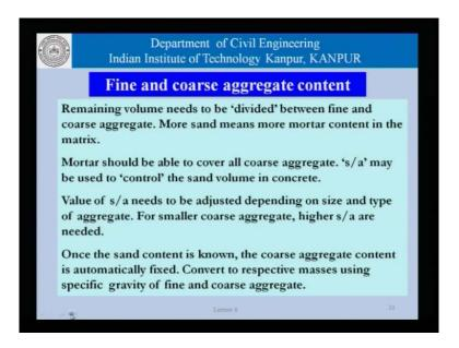
So, we will work with those examples as we go along in this discussion now as far as the determination of fine and coarse aggregate is concerned, what is the crux of the problem? The remaining volume needs to be divided between the fine and coarse aggregates, more sand means more mortar content in the concrete or in the matrix and less sand means less mortar.
