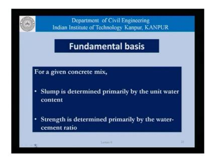
We said that slump or workability of concrete is determined primarily by the unit water content and that depends also on the type of materials being used. Then, the strength is determined primarily by the water cement ratio, so with these two assumptions we actually gets started and carry out the exercise of proportioning concrete mixes.
