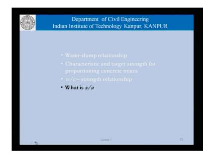
Now, coming to the last item, that we have for the discussion today as a concept in proportioning concrete mixes is the s by a. That is the sand to aggregate ratio or the sand in the aggregate ratio.
