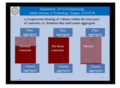
So, if we have s by a representing the sharing of volume within the inert part of concrete, that is between the fine and coarse aggregates, then if we have normal concrete like this where there is a reasonable amount of fine aggregate, a reasonable amount of coarse aggregate in the system. If we have very low s by a, we have a no fines concrete and if we have a very high s by a, we are virtually working towards mortar.
