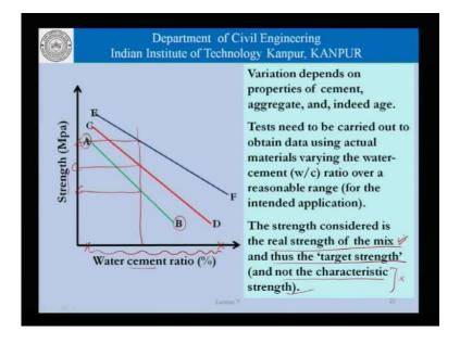
Now, let us come to the next concept which is the water cement ratio versus strength relationship, much like the discussion that we had in terms of the unit water content and the slump. Here too we have a variation of water cement ratio and the strength of concrete, which could be the compressive strength of concrete determine using queues or cylinders. We can have a variation a b and again to simplify things, we can connect
