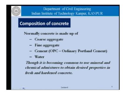
We also have gone through the constitution or the composition of normal concrete, which consist of course, aggregate, fine aggregate cement and water.
