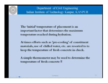
The initial temperature of placement is an important factor that determines, the maximum temperature reached during hydration. At times efforts such as pre-cooling of constituent materials, use of chilled water and so on are resorted to keep the temperature of fresh concrete in check because there may be specifications, which say that the
