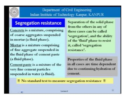
Now, let us come to segregation resistance which is a slightly different property concrete we know is a mixture comprising of coarse aggregates suspended in mortar. Mortar being a mixture comprising of fine aggregates suspended in a fluid phase of cement paste, and a cement paste itself is a mixture of very fine cement particles suspended in water, which is a fluid.
