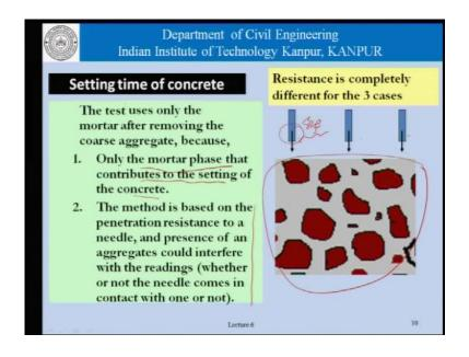
When we are doing setting time for concrete, when we are trying to do the setting time of concrete or measure the setting time of concrete, we said that the concrete is wet sieved to remove the coarse aggregate. Now, the logic for that is given here, it is only the mortar phase that contributes to the setting of concrete. Coarse aggregates their presence does not really affect the hydration process.
