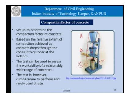
Continuing from there let us talk of the compaction factor test basically, what this test does is allows the concrete to fall from one container to another and then to another. And we compare the density of the concrete obtained here, with respect to another density which is obtained by filling the same container, and compacting the concrete using vibrators and so on. So, that we get the maximum possible density.
