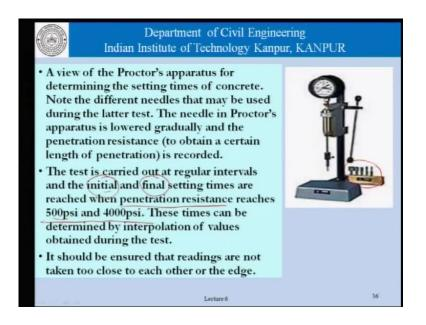
Concrete sets overtime, as a result of the formation of more and more hydration products, during hydration. Now, we are familiar with the setting of cement and we know the initial setting time, and the final setting time of cement is a quality control parameter. And we have specifications which say, that the cement should not have a initial setting time higher than something or lower than something, it should not have a final setting time, which is higher than something or lower than something.
