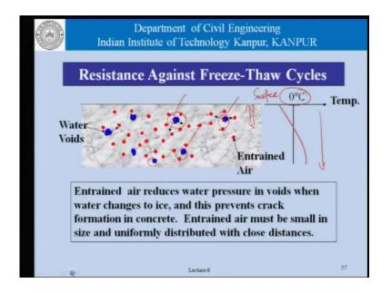
When it comes to the resistance against freezing and thawing, what we are trying to do really is to see how these air particles help, in dissipating the forces that will arise or the pressures that will arise, when these water voids or these voids full of water. The water in these voids tends to freeze on account of a temperature in the atmosphere, which may go below 0.
