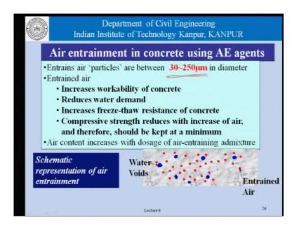
So, really speaking air entrainment does not necessarily lead to a net reduction in strength, but in principle yes, as we increase the air the strength tends to go down. Now, taking a closure look at the air entrainment concrete using air entraining agents, these particles are in the range of about 30 to 250 micrometers and diameter, and they set in a concrete matrix much the way this these red dots are shown. And there are water voids which are all over the place and so on.
