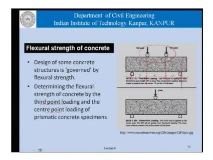
When it comes to flexural strength, which again is required in certain structure which are governed by flexural strength. The ASTM for example, gives us the alternative of the third point loading or the center point loading. The third point loading basically, says that we have a prismatic beam and we apply the load at two places on the top, and these three spans are equal.
