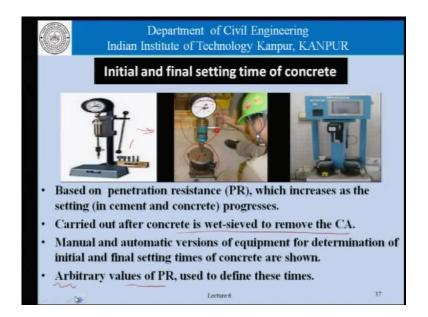
The test is carried out at regular intervals, we try to study the penetration of these needles, and once the penetration resistance reaches a level of 500 PSI, and 4000 PSI. And leaving in the conversion to the SI units out of here, please do it at your end, and when the penetration resistance reaches these levels, we say that the concrete has reached initial set and final set. The initial set corresponds to a penetration resistance of 500 PSI
