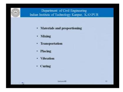
As far as stages in concrete construction is concerned, we had laid out materials and proportioning, mixing, transportation, placing, vibration, and curing.
