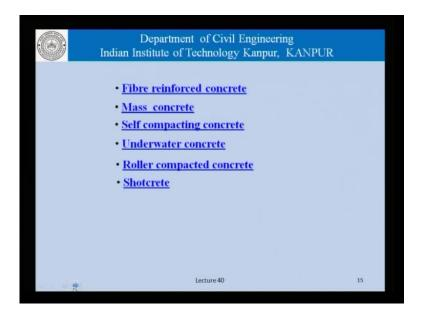
As far as special concretes is concerned, we had laid out, fiber reinforced concrete, mass concrete, self-compacting concrete, underwater concrete, roller compacted concrete, and shotcrete has some examples of special concrete; based either on the use of materials or the conditions of placement, and method used in placement, the environment of placement, method in vibrating the concrete, and so on.
