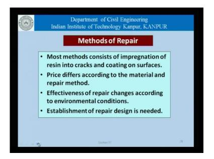
Now, as far as the methods of repair are concerned most methods, consists of impregnation of resins into cracks and coatings of surfaces as far as concrete is concerned most deterioration manifest in the form of appearance of cracks of some nature or the other and therefore, the and therefore, repair action is basically impregnation of resins into these cracks, and then applying coatings on the surface.
