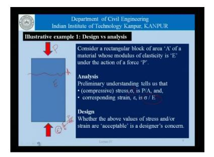
Now, let us extend our discussion to include the concept of design versus analysis. Consider a rectangular block of area A of a material whose modulus of elasticity is E under the action of load P. So, what we are talking about that the load P acts on this block of material which has an area of cross section A that the material property is E the modulus of elasticity of this material is E.
