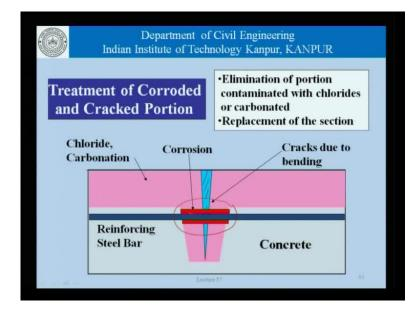
Now, this here is a representation of treatment of corroded and cracked portions in a concrete structure, corrosion being a most common cancer as far as concrete structures is concerned, if this is the portion of reinforcement which shows corrosion in the neighborhood of a crack what we would like to do is to eliminate portions contaminated with chlorides or portions which are carbonated and then replace the material there with something else as shown in this section.
