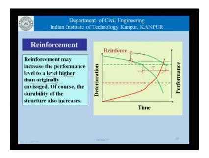
Now, what is the reinforcement action? Reinforcement action means increasing the level of performance to a level which could be higher than the originally envisaged level and of course, the durability of the structure also increases. Now this is explained here that if we decide to take reinforcement action at this point in time, because of our action the performance level has increased and not only it has increased may be the slope it which it was deteriorating has also been rectified.
