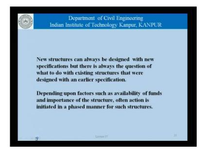
Now, new structures can always be designed with new specifications but, there is always the question of what to do with existing structures that were designed with an earlier specification. A structure which was designed with the certain specification may continue to perform as design but, due to changes in specification that response or that performance becomes unacceptable.
