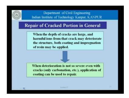
If we talk about repair of crack portions in general, if the depth of cracks is large and is harmful from the point of view of corrosion and so on. We may choose both costing and impregnation and if the deterioration is not so severe, it just cracks on the surface not very deep, we may choose to apply only the coatings on the surface but, these two coatings now need to be different qualitatively as we shall see.
