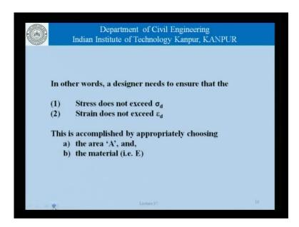
Now, what is the design? Correspondingly the design means, whether these values that is sigma that we get here or the epsilon or the strain that we get here, these are acceptable or not; in other words the designer needs to ensure that the stress does not exceed sigma d which is what we have determined earlier and the strain does not exceed epsilon d. How does it done?
