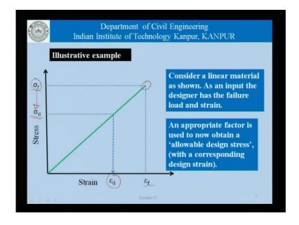
Let us take an illustrative example as to how the design process really works. Here is the stress strain curve of a linear material and as an input; the designer has the failure values here. The failure stress and the corresponding failure strain. Now what we really do is an appropriate factor is used to obtain an allowable design stress with a corresponding design strain.
