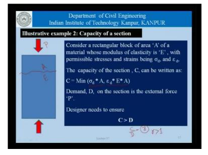
Now, this concept of enough capacity basically, means that the capacity that is a supply should exceed the demand by a certain margin. Going back to this example, that we had of a rectangular block with area A modulus of elasticity E and the permissible stresses
