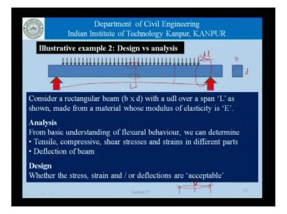
So, let us consider another example. Here is an example of a simply supported beam measuring d by d, that is the cross section of the beam and it has a uniformly distributed load over this span L. Assuming that the modulus of elasticity of the beam is E. The analysis means that from the flexural behaviour of the beams. We determine the tensile, compressive, shear stresses and strains in the different parts of the beam. We know that
