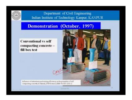
Compared to that, if we use a self-compacting concrete mix, more or less the surface that we get is horizontal except that, it is not truly horizontal. And the level or the extent, to which the surface deviates from the horizontal, is actually a measure of the selfcompactability of that concrete.
