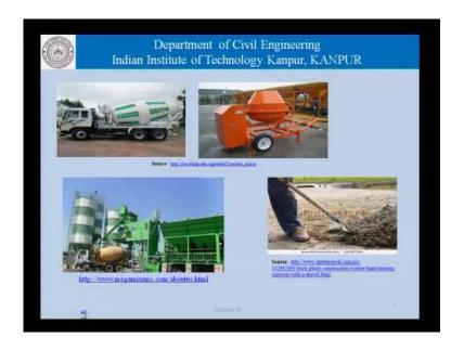
Another kind of mixing that goes on in concrete construction and we must be aware of that is when the concrete is being transported from the batching plant to the construction site and that mixing is in advertent, because the intension of that process in an agitator truck is not really to mix the concrete unless is so designed but basically to keep the concrete agitated and ensure that the concrete does not set.
