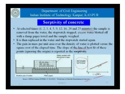
This here is the test for sorptivity of concrete that is a relatively new test which were a concrete specimen, which is 100 mm diameter, 50 mm thick is exposed to water with the filter paper raped on it. And it is selected intervals ranging from 1 to 25 minutes, the sample is removed from the water stopwatch is stopped, so we are watching or we are measuring the penetration of water, or they absorption of water by this is specimen, in a matter of minutes.
