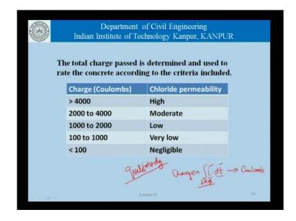
What is really done at the end of it is, the total charge passed is determined, because the charge, the charge that is passed is related to the current it is a only the integral of the current water time for the whole of 6 hours, and this is measured in coulombs. Once we have the i and t data that how much of current is flowing through the two faces or through the concrete, over a period of 6 hours at periodic intervals, we can convert and obtain the total charge that has passed.
