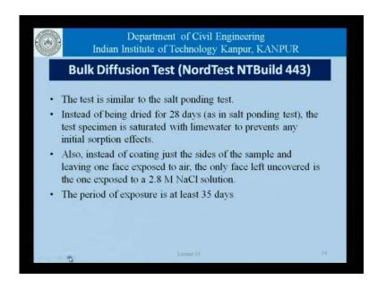
Continuing the discussion on chloride permeability, there is a bulk diffusion test, call the Node Test NTBuild 443, and this test is basically similar to the solve ponding test, except that instead of being dry for 28 days, the test is specimen is saturated with lying water, to prevent any initial option effect. And also instead of coating just the sides of the sample, and leaving one face exposed to air, the only face left uncovered is the one
