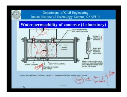
So, in principle what we have is a lot of methods use a setup, which is summarized here, we have a concrete specimen, on one side we have chloride reach environment, on the other side we have a environment which is not having chlorides to begin with. And then we try to push the chlorides through the concrete on to the other side, now if we apply a direct current here, the test becomes similar to or the test basically becomes the T277, that is rapid chloride permeability test.
