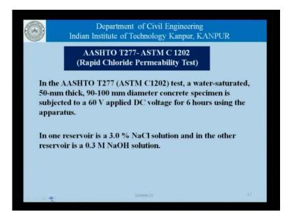
One of the tests that comes to mind in this contexts, is the AASHTO, American association for state an high way transport officers, there test standard quality T277 or the ASTM is C1202, which is a rapid chloride permeability test. Now, this as the name
