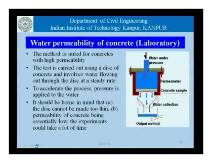
Now, let see what the water permeability of concrete the so called output method or the constant had method means. It means that first of all the method is suited for concretes which are highly permeable, that is a concrete sample which is place like this, and water is put here, and a pressure is applied, water actually flows out from the other side of the concrete sample. And we can collect a certain reasonable amount of water, in a reasonable time frame.
