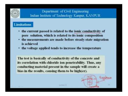
This test obviously has certain limitation; the current past is related to the ionic conductivity of the pore solution, which is related to its ionic composition. What is happening in this test is that at the end of it, this is the concrete piece or the specimen, and we are applying a charge, which causes this current to flow through the concrete. So, even though we are trying to measure the current, what we are effectively trying to do is to determine the resistance of the concrete.
