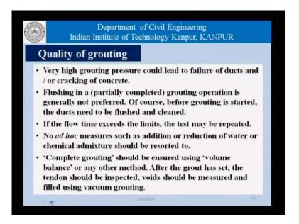
As far as the quality of grouting is concerned very high grouting pressures could leads to failures of ducts and in cracking concrete. Flushing in a partially completed grouting operation is generally not preferred. We cannot stop the grouting operation and then, try to flush it out and then, commence again because of the obvious reason that the flushing may not ensure all the removable of grout and that would become a problem if you want to go back again and grout a system.
