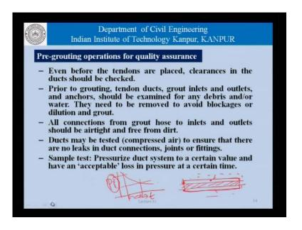
Prior to the grouting, tendon ducts, grout inlets and outlets and anchors whatever they are should be examine for any debris and or water. They need to be removed to avoid blockages and or dilution of the grout.
