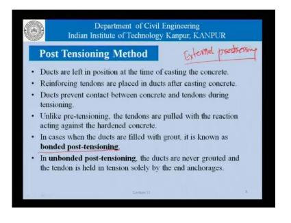
As far as the post tensioning method is concerned: the ducts are left in position at the time of passing the concrete, reinforcing tendons are placed in the duct after the concrete has been cast, the ducts prevent contact between the concrete and the tendons during tensioning, unlike pre-tensioning the tendons are pulled with reaction against the harden concrete and that is why we need a certain amount of strength in the concrete before the tensioning can be done.
