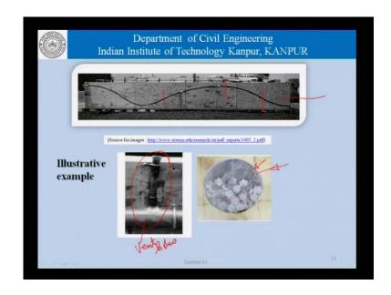
Now, this here is an illustrating example taken from one of the references. So, the prestress tendons are not necessarily straight and they could follow the profile which sometimes looks like this. And these here are vent holes which help us remove the air from the duct while the grout has been moved in and then of course, we can try to take pictures of cross sections at different places and try to see whether or not the duct has been fully filled with grout.
