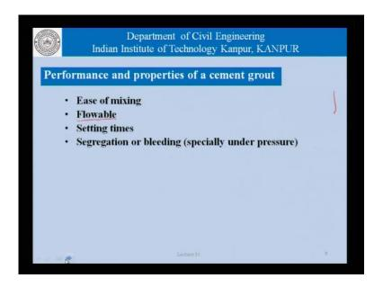
Segregation or bleeding specially under pressure. Grout like any cementitious composite that we have talking about tends to bleed. That is, water tends to separate out from the constituent materials and this tendency for segregation is sometimes enhanced when the material is beam moved under pressure. So, to have to be able study or we should have a bench mark on what is an acceptable level of bleeding.
