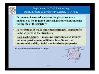
Now, coming to special from works. Let us first talk in terms of what is called permanent formwork. Temporary formwork is the normal formwork which is removed after the concrete has achieved sufficient strength. Permanent formwork on the other hand contains the placed concrete, molds it to the required dimension and remains in place for life of restructure. That is, this formwork is not removed after the concrete has been cast it becomes part of the concrete remember itself.
