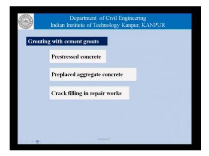
Now, coming to the applications of cement grout as for as civil engineering is concerned. One of them is in pre stress concrete, the other reason preplaced aggregate concrete and the third is crack preliminary repair works besides several where applications which are not traditionally which are not really in the embed of concrete engineering. Coming to pre-stress concrete, we had talked about at sometimes that there are 2 kinds of prestressed in concretes.
