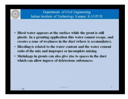
As far as bleeding is concerned, bleed water appears at the surface while the grout is still plastic. And in a grouting application this water cannot escapes and there is no way that
