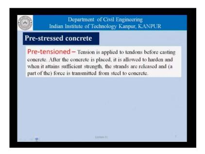
One is pre-tensioned where, tension is applied tendons focused in a concrete and after the concrete is placed it is allowed to harden and when it attains sufficient strength, the stands are released that is, the tension in the stands is then transferred from the steel to the concrete or at least a part of it is transferred the concrete and by that token the tension in this steel tendons reduces is to some extent. Coming to post tension systems
