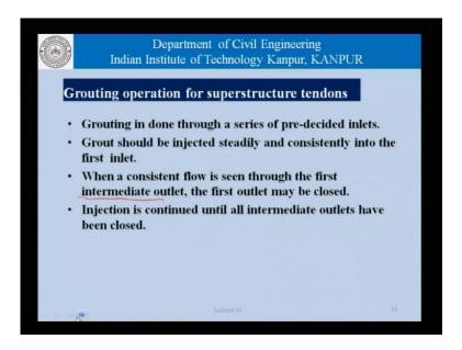
When a consistent flow is seen through the first intermediate outlet. So, there are series of outlets and we are trying to pump the grout into the first outlet and as the grout immerges in the second outlet of the first into which is outlet the first outlet can be closed and then we used the second point as the inlet to push the grout further and this processes carried on till all the grouting completed. As we say here injection is continued until all intermediate outlets have been closed.
