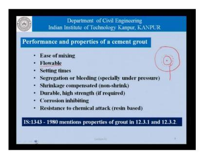
Durability and strength are obviously requirements in any cement based construction and grouting in post tension concrete, ducts is no acceptation we need or we made specified that for the grout that we will use it is the certain strength at a certain point time whether it is 28 days of 7 days or 3 days or whatever the time being.
