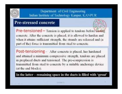
In this case after the concrete placed it has harden tendons has obtained how many minimum compress strength, tendons are placed in preplaced ducts and tensioned. So, basically the ducts are already in place at the time when the concrete is casted. The precompression is transmitted from the steel to concrete by a suitable anchorage device at the end blocks. So, this is the principle of post tensioned concrete.
