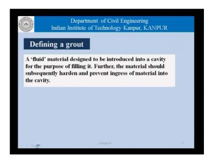
So, now starting the discussion with grouting. What is a grout? It is defined or it can be defined as a fluid material designed to be introduced into a cavity for the purpose of filling it. Further, the material should subsequently harden and prevent ingress of deleterious material into the cavity.
