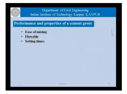
Another property for the grout which would be of interest was is the setting time. Like all concrete construction, the grout once it is re-stress final location we would like the system to set and therefore, the setting time is of great importance as far as grouts are concerned.
