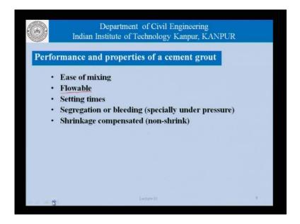
Shrinkage compensated - Again, grouts because they do not have cores segregate. Proportionally speaking the volume of cement is much higher and therefore, there is a tendency for the grout to shrink unless special measures are taken to admixtures so on. To make and design shrinkage compression grouts that is non-shrink out do not have which do not shrinkage.
