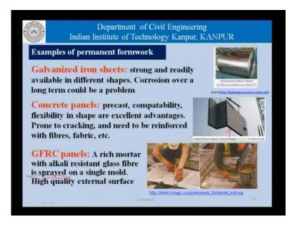
Other materials as far as permanent formwork is concerned could be galvanized iron sheets which are strong in readily available and different shapes. Corrosion over a long time could be a problem in the case of using sheets in therefore, we need to be careful as to what kind of tests are carried out to ensure the durability of these sheets. Concrete panels which are pre casts, highly compatible with concrete construction.
