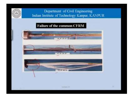
Another thing, which we will see later on in the next slide perhaps. This slide here shows the failure of the common CFRM; the aramid fibers, the carbon fibers, the glass fibers and in all cases we see that there is a fair amount of delamination's that has occurred, fibers have become separated from the matrix, the matrix has completely collapsed and so on. One thing I would like to point out when testing CFRM is the role of these anchors at the end of the specimens.
