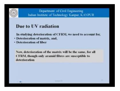
As far as ultraviolet radiation is concerned we have to account for of course, the deterioration in the matrix and the fiber. And, what most experiments of the studies are found that the deterioration in the matrix of course, will be the same. But only for aramid fibers there has been some reported deterioration as far as the change in strength on account of the exposure to ultra violate rays is concerned.
