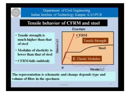
Now, comparing it once again as far as steel is concerned, then what it looks like. For carbon, the modulus of velocity is about one-third that of steel and the biggest difference is that we have a large fracture load but we do not have any capacity in terms of deformations is concerned. The deformation is brittle; it does not allow us any warning, there are no large deformations possible and that is something, which we must be keep in mind when we are designing structures using CFRM.
