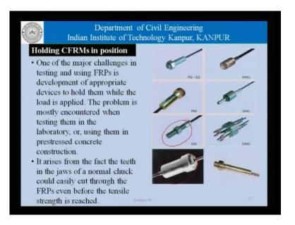
So, designing these devices or these anchorages is a technological challenge as far as FRP's are concerned, their use in the field in the post stationed, pre-stress construction is concerned.
