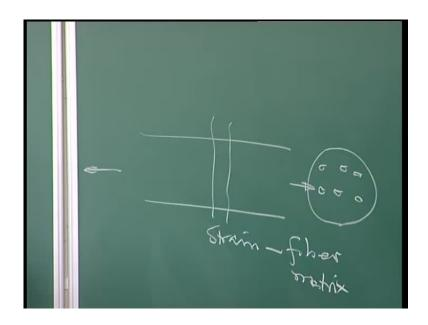
What we are saying is that if we take a CFRM, which is like this, with the lot of fibers and we apply the load in this direction. Then, the strain that we see here, whether it is in the fiber or it is in the matrix; it is the same and that is the value that we have for the composite itself. And under those conditions if we apply simple rules of stress and strain, we will get the equations which are given here.
