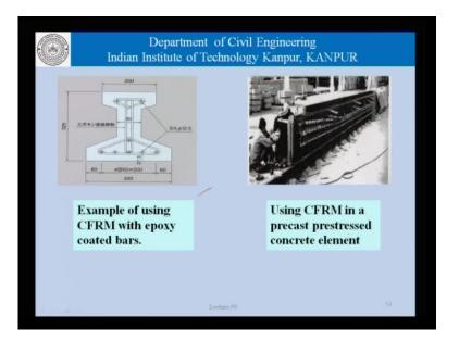
Continuing with the examples, we have CFRM with epoxy coated bars in the case of girders which is shown here. In this case as well as in a pre-stressed, pre-cast concrete element has been shown here.
