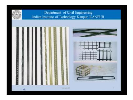
And, then we had seen this picture which is the products from the long fibers. And, we can see that they are in the form of rods, strips, 2 dimensional, 3 dimensional, woven into nets, fabrics and so on and so forth.
