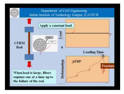
This picture shows the representation of a creep test using CFRM rods. What is done is that a CFRM rod is held in position at a constant load; that is the load is held constant over a period of time. Now, depending on the load level, there will be a certain amount
