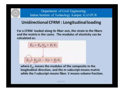
That is E c l will be equal to E m times V m plus E f times V f; which can be written as, because the volume of the matrix is nothing but 1 minus v volume fraction of the fiber as
