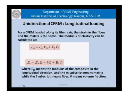
Now, as far as the unidirectional CFRM and that is what we are really bothered about is concerned in the longitudinal loading; for a CFRM loaded along its fiber axis, the strain in the fibers in the matrix is the same.
