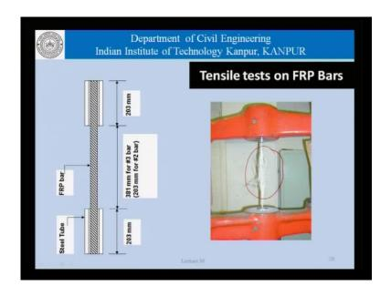
This picture here shows the tensile tests on FRP bars. So, if we look at the tensile test, this is how the FRP bar fails. So, it is a very brittle failure, destructive in nature and does not give us any time as far as the netting is concerned. So, there is absolutely no large deformation region.
