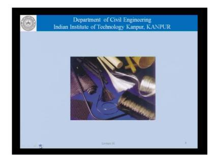
And, these are the pictures that we have seen this is the different fibers; carbon, glass, aramid, in the raw form; that is the fibers themselves which are extremely fine.
