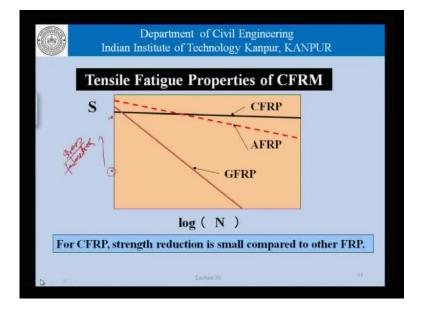
Now, this is represented traditionally in the form of an S N curve which really shows that the number of cycles to failure at a certain stress level. So, this level here on the y axis is the applied stress to the failure stress. So, if we are going higher up in this picture here, we are moving in a manner where the applied load level is closer to the failure stress. Whereas, the stress here is lower than the failure stress.
