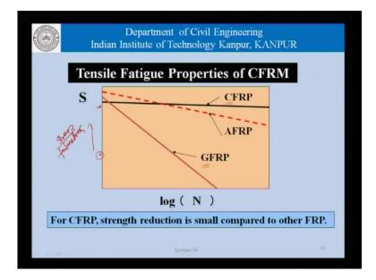
And, that is what is represented by these two points here along the y axis and naturally if the stress levels are lower and naturally if this stress levels are lower, the number of cycles to failure or higher. And, if the stress levels are higher, the number of cycles to failure is low. And, if we study this S N curve for the different fibers, we find that the glass fibers are most vulnerable as far as fatigue loading is concerned. Comparatively, the carbon fibers show much better performance.
