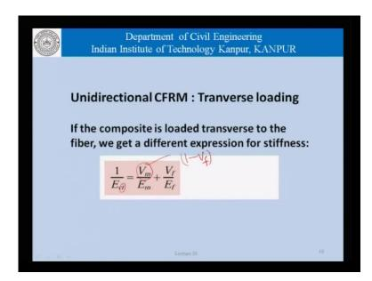
Similarly, if the load was applied in the transverse direction that is in a direction perpendicular with the orientation of fibers we are not doing the derivation here. But the E transverse; so, this t here is transverse. So, the E transverse of the composite can be written in terms of V m upon E m plus V f upon E f and we can write V m as 1 minus V f like we had done in the previous case.
