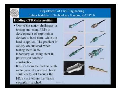
One of the major challenges in testing and using FRP's is the development of appropriate devices to hold them in position while the load is applied. The problem is mostly
