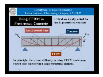
And, there is no reason why CFRM cannot be used with traditional reinforcement or epoxy coated bars and so on in RC members or pre-stress concrete members. And, given their high strength the CFRM or an ideal material for use in pre-stress concrete as I shown here. So, this tendon here which is going to be used for pre-stressing could be a CFRM and the other reinforcement is simple epoxy coated bars or normal bars whatever we want.
