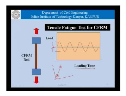
Basically, this level here how high or how low is this level compare to the failure level. If this is the stress strain curve of the material and the applied load is being varied at this point versus the applied load is varying at this point; this here is at a lower stress level and this is at a higher less stress level.
