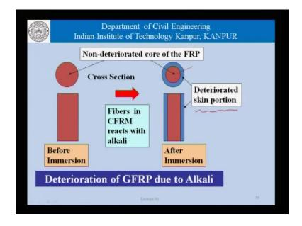
As far as a model is concerned we can look at it the way it shown here, that there is a deteriorated skin portion; that can be identified as far as a glass FRP is concerned. And, only the core remains unreacted or undamaged. One of the ways therefore, to use glass reinforced fiber plastics in concrete construction would be to have a coating on the glass fibers and the CFRM in order to protect them from reaction of alkalis in the environment.
