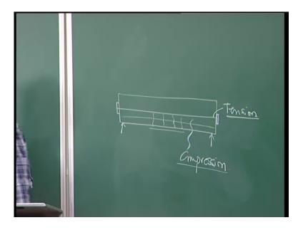
When we have a beam and it deteriorates (No Audio From: 39:17 to 39: 26). If there is a concrete beam with reinforcement which has cracked; one of the ways of repairing this beam with external reinforcement would be to just have something outside this beam and tie the two ends using something like a fiber reinforced plastic rod. And, if we introduce
