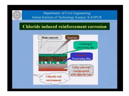
And we talked about the reasons. why that does not happen, the reason is the formation of this passivating film in the neighborhood of the reinforcing bars, because of the high p H of the pore solution and concrete which is a product of the formation of large amounts of calcium hydroxide on account of large amounts of calcium hydroxide which is formed when cement hydrates.
