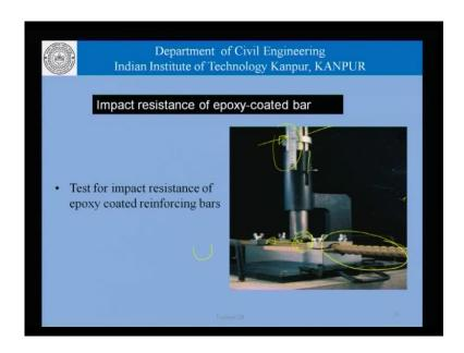
Let us say that it 15 centimeters the performance is acceptable that is the coating does not get damaged, at 16 centimeters again it is acceptable so long as it is acceptable. We increase the height to determine what happens at that next stage? So for example, it is 17 is also acceptable. But at 18 the performances not acceptable, what is done actually is that we need to keep changing the location as well, what we need to do is to keep changing the location at which the straight occurs.
