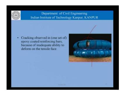
Is being left out from our discussion today, now this picture here shows what happens to a bar which is not good enough. This picture here shows that the cracking; this picture here shows that the coating has cracked it has simply failed it did not have the right amount of flexibility. And when the bar was bend there was a failure at this point compared to the bar shown below.
