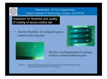
So, at the end of end the cost is very important parameter that we must in mind when we are using any new material. Coming to other methods there are test for flexibility and quality of coating of epoxy coated bars. So, this picture here is that for flexibility of a coating, whereas this picture here is a visual inspection of the coating on the reinforcement bar.
