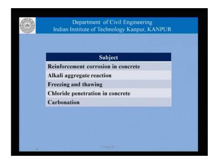
Now in this we are talked of mechanisms of deterioration in concrete structures.
