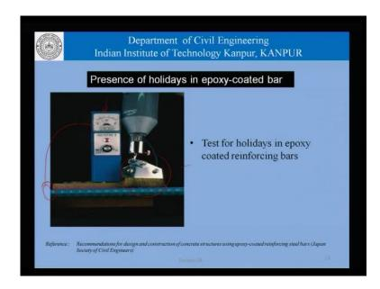
So, this is the bend test for the epoxy coated bars. This device here is used to detect to presence of holidays or pin holes in epoxy coated bars. And as was mentioned earlier
