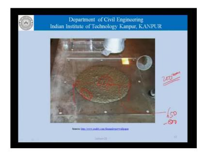
What we are really talking about is that this diameter here, which is what the concretes spreads into once the slump cone has been removed, this should be of the order of 650 to 800 millimeters or 600 to 850 millimeters. The original diameter here as when it was
