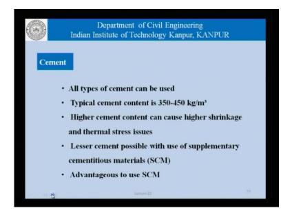
Now, we use a land up using a lot of these cementitious materials in self-compacting concretes for the simple reason, that we need to have higher volume of paste higher
