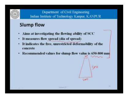
What we must remember is that the standard slump cone, measures a 100 millimeters on the top, 200 millimeters here, and has a height of 300 millimeters. So when we are talking of a slump flow of 650 to 800 millimeters;
