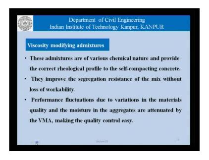
As far as the viscosity modifying admixtures are concerned these are of various chemical nature, and provide or correct desired rheological profile to the self-compacting concrete, they improved the segregation resistance of the mix without loss of workability, they also help to reduce performance fluctuations due to variations the material quality. And the moisture in the aggregates this helps us maintain a consistent quality as far as self-compacting concretes are concerned.
