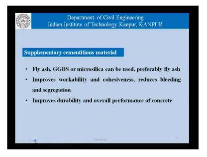
As far as these materials are concerned we could use fly ash, the blast furnace slag or microsilica, preferably fly ash because of its spherical nature they use improves a workability and cohesiveness, reduces bleeding and segregation, improves durability and overall performance of the concrete.
