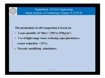
So, it is these three principle factors or a combination of these factors which helps us obtain self-compactability in concrete. So, when we are talking of a large amount of fines we can imagine that if you are looking at 500 to 650 kgs per cubic meter fines, this is not including the fine aggregate, this is really the fines in the sense of cement and particles which are of similar size.
