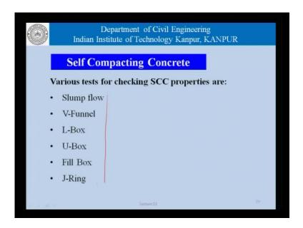
Some of the test that we will talk about today are the Slump flow, the V-Funnel, the L-Box, the U-Box, Fill Box and the J-Ring. Now, these tests give us an entirely different framework in which a self-compacting concrete can be evaluated; we must remember that self-compacting concrete has been developed only about 25 30 years ago and therefore, a lot of these tests are still in some form of development or the other.
