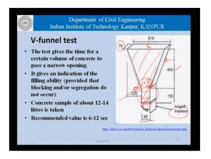
Now, if we come to the V-funnel test. The test give us the time for a certain volume of concrete to pass through a narrow opening; it gives an indication of the filling ability provided that no blocking, and or segregation occurred, concrete samples would depend upon the size of the V-funnel; it could be about 12 to 14 liters, and the time would vary between 6 and 12 seconds.
