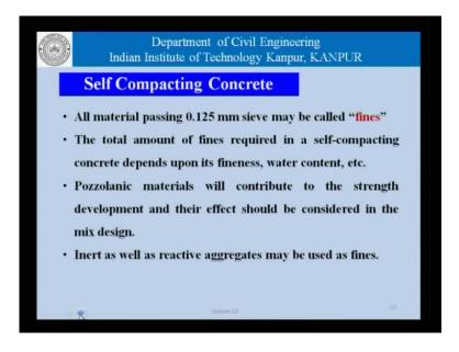
So, we cannot obviously have this amount of cement sitting in a concrete matrix so, the cement content has to be restricted to about 350 to say 450 and therefore, perforce or by
