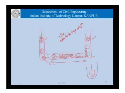
So it is a variation of the U-Tube test, that we talked about except that concrete is just not flowing from one leg of the U to the other, but it is passing through or reasonably long distance. Now, as this concrete goes through this distance, we can always have innovations which would create obstacles in the path of the flow, and still expect the concrete to negotiate the barriers that we put in place.
