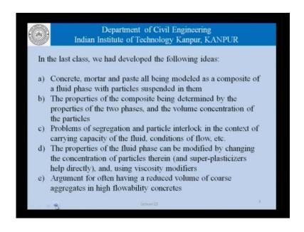
Concrete mortar and paste all can be modeled as a composite having a fluid phase with particles suspended in them, paste can be modeled as cement particles suspended in water, mortar can be modeled as sand particles suspended in paste, and concrete can be modeled as coarse aggregate suspended in mortar.
