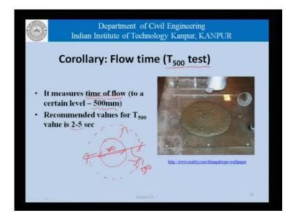
As a corollary to the slump flow test, we also sometimes use a flow time which is sometimes called the T 500 test; and now this T 500 refers to the time, it takes for a concrete to achieve or reach a diameter of 500 millimeters, and the typical time could be in the range of 2 to 5 seconds.
