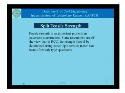
Tensile strength is an important property as far as pavement construction is concerned, and some researchers after view that in RCC, that is when using roller compacted concretes. The strength should be determined using course, where we determine this split tensile cylinder, and not necessarily from the flexural test of beams. Now, the reason for that is something which I would like to leave to you to ponder about.
