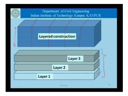
Instead we divided the block in layers, and caused this as layer 1 followed by layer 2 and finally, followed by layer 3, so this a fundamental difference between casting this large block with blocks, which is like this or in terms of layers which is like this. Now, what
