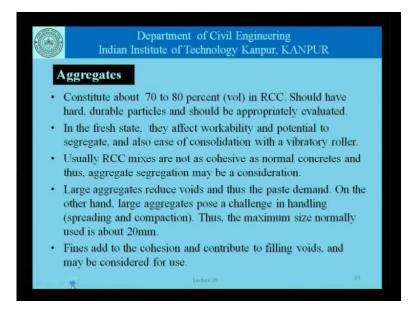
Now, the ingredients are not different from normal concretes, accept that in the case of RCC, the aggregate constitute about 70 to 80 percent by volume, and naturally they should be hard durable particles, and should be appropriately evaluated. Appropriately evaluated means, we already have that test to carry out evolution of aggregates, in terms of the physical properties. And those tests are no different simply because they aggregate
