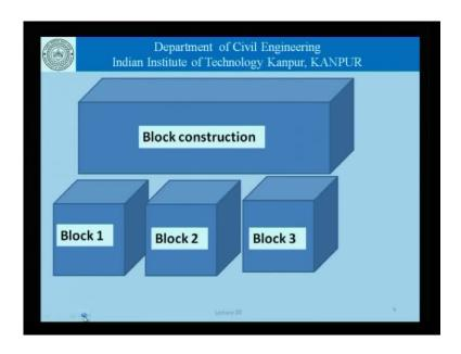
And these three blocks are caused one after another with the suitable gap and so on, and so forth; that is one way of casting this large concrete block. Another possibility could be that instead of blocks, we talk in terms of a laid construction, in which case we divide this block not as blocks like we did last time that is this way, we do not do that.
