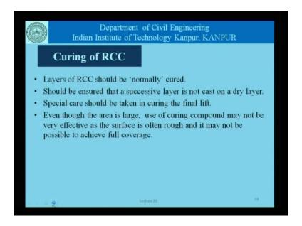
Now, coming to curing of the RCC, the layers of RCC should be normally cured that is there is no reason to believe that the curing can be done, or needs to be done any different layer. It should be ensured that successful, if layer is not caused on a dry layer of concrete, because as it is the amount of water present in a concrete is less. And if that water to gets absorbed in previously cast lift it is likely to lead to a poor quality construction.
