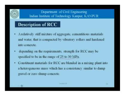
And due to that reason, in the fresh stage it looks very different, the constituents materials for RCC are blooded in a mixing plant into heterogeneous mass, which has the consistency, similar to damp gravel or zero slump concrete. So, the basic principle or of concrete engineering is not violated, we still have the same materials that is aggregate cementitious material, that is cement and the fly hash and water.
