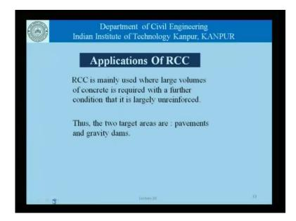
Now, continuing with the applications, it is mainly used where large volumes of concrete are required with the further condition, that the concrete is largely on reinforced. The presence of reinforcement makes the placement of concrete difficult, and adds a very different dimension to the casting. And therefore, as for as roller compacted concrete is concerned, attention is generally confined top plain concrete.
