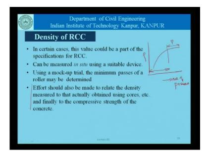
We did talk about density a little bit, and in certain cases this value could be the part of the specifications of the RCC, it can be measured is to using a suitable device, and using a mock up trail the minimum passes of a roller may be determined. So, in a mock up that precedes actual construction, we may determine or estimate that in order to get a certain density of the concrete, what is the number of passes that are required.
