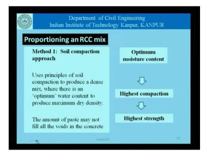
Now, here given the very special method of compaction, sometimes we use the soil compaction approach to proportion of RCC mix, which is different from our traditional method of proportioning concrete mixes which we have practice so far. In this case what we do is use principles of soil mechanics, and soil compaction to produce a dense mix, where there is optimum water content to produce maximum dry to density.
