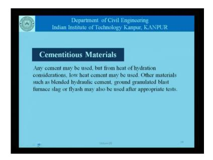
Fines add to the cohesion of the concrete and contribute to filling the voids and therefore, should be considered for use. As far as cement issues materials are concerned any cement can be used, but from the point of view of the heat of hydration use of low heat cements, may be considered. Having said that, we should remember that roller compacted concrete is after all being placed in relatively thin layers, and thermal stresses are not likely to be a major problem.
