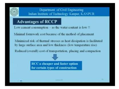
And as far as the advantages concerned, we have low cement consumption, because the water contented self is very low, we have minimal formwork cost, because the method of placement as we good see, that there is hardening form work required, except at the (( )). There is a minimized risk of thermal stresses as heat dissipation, is facilitated by the large surface area and smaller thickness which means, there is low temperature rise and virtually low thermal ingredients.
