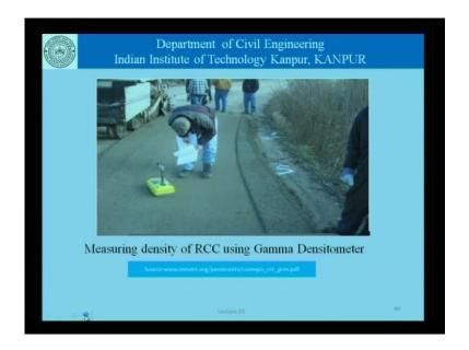
Now, this here is the measurement of density of RCC or the in situ measurement of density using a gamma density of meter.
