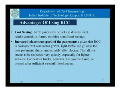
As far as the cost saving is concerned, the RCC payments, if we are may be if we are making pavements or rods using a roller compacted concrete, we do not use doubles and still reinforcement of forms, and this results in significance savings. As far as the increased placement speed is concerned that helps us a lot, this couple with the fact that RCC or roller compacted concrete can be looked upon as basically wet compacted gravel.
