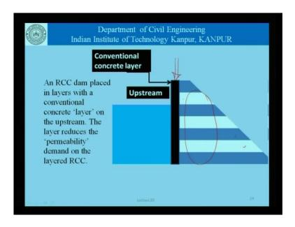
However, if the concrete was caused in a manner that this layer, or this lift of concrete along the height of the dam is caused with conventional concrete. That is it is not caused in layers as shown here, in that case we are not so much bothered about the permeability of the roller compacted concrete.
