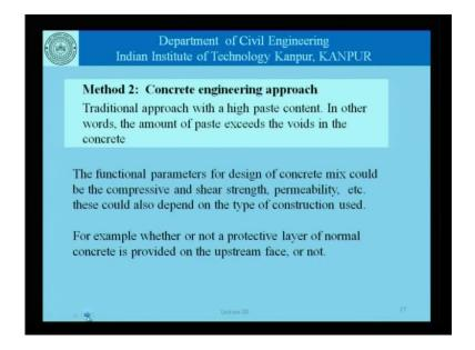
Now, as against this we of course, have the concrete engineering approach where the paste content is high, high paste content means the amount of paste exceeds the voids in a concrete. And that is the traditional approach that we are already know that we have the water content, that we have the cement content, we make sure that the paste content is hard then the void content, and proportion the mixing so on.
