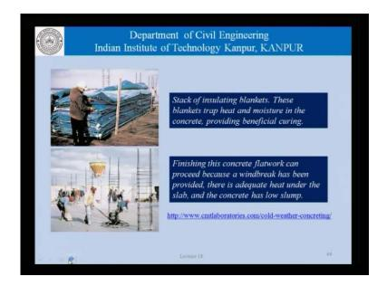
The picture on the top here is a stack of insulating blankets. These blankets trap heat and moisture in the concrete and provide beneficial curing. The errection of these kinds of wind barriers helps us protect the concrete slab which has been cast here and enable us to carry out the finishing operation. In this case of course, the silver lining in the cloud is
