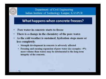
What happens when concrete freezes? Pore water in concrete starts to freeze. There is a change in the chemistry of the pore water. Because, once part of the water is frozen, part of the water is not, the concentrations of the ions in the different parts of water are
