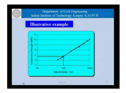
What is really done is, we calculate the maturity of concrete which is the sum of a temperature component and the time component. And once we have this maturity, we try to relate this maturity to the compressive strength. T 0 here, is a datum temperature, which is the reference temperature, which is taken as minus 5 or minus 10 degree centigrade.
