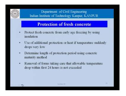
It needs to be protected from early age freezing by using insulation. We need to use additional protection or heat, if temperature suddenly drops very low. We need to determine or estimate the length of protection period using maturity. Maturity is a concept as we will see later, which integrates the time and the temperature.
