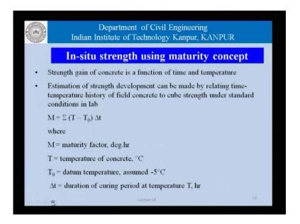
Now, explaining the concept of maturity which we have related to the previous discussion just now. The strength gain in concrete is a function of time and the temperature. The estimation of strength development can be made by relating the time temperature history of field concrete to cube strength under standard conditions the lab.
