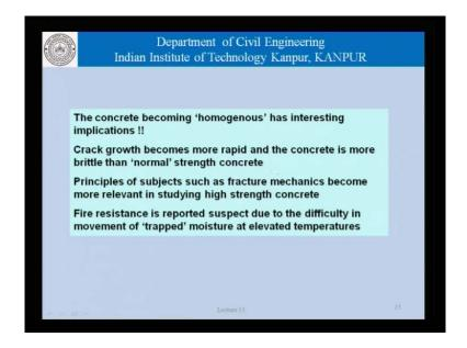
The principles of subjects such as, fracture mechanics becomes more relevant in studying high strength concretes. Fracture mechanics is the science that studies crack formation crack propagation and so on. If you read the literature on fracture mechanics you will realize that the whole assumptions, the whole set of assumptions made in fracture mechanics are more valid when we are talking of high strength materials, more homogeneous materials within concrete than normal concrete.
