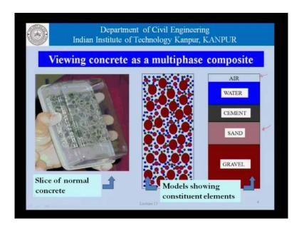
Now, this slide we have seen before. It is again viewing concrete as a multiphase composite which shows that, if we take a slice of normal concrete, what we see is that, concrete can be looked upon as aggregates or well course aggregates embedded in a system of mortar.
