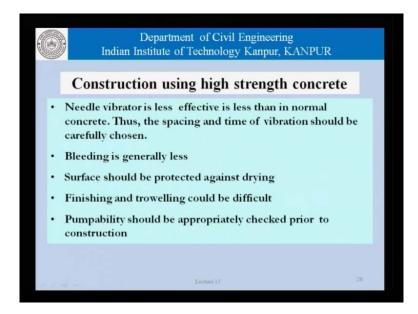
When it comes to construction using high strength concrete, we must remember that the concrete is now characterized by the presence of a large amount of paste or a large amount of mortar which makes the concrete very viscous. And once the concrete has become viscous then, needle vibrators are less effective than in the case of normal concrete. And therefore, the spacing and the time of vibration needs to be carefully chosen.
