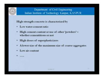
Now, what are the characteristics of high strength concrete? High strength concrete is characterized by low water cement ratio. Naturally, unless we lower the water cement ratio, the water that is available beyond that required for hydration of cement cannot be controlled and that excess water is the one that is responsible for the creation of pore spaces.
