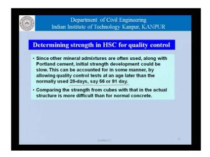
Now, let us talk a little bit about determining the strength for high strength concretes. As far as quality control is concerned. One thing that comes to mind is the age at which the quality control should be carried out. Since, mineral admixtures are often used along with Portland cement, strength development at least in the initial part could be slow. And this could be accounted for in some manner by allowing quality control test at an age later than the normal 28 days, say 56 or 91.
