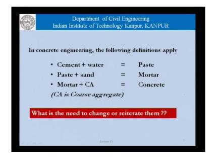
This again is just definitions which we have seen before. Cement and water is paste; paste and sand is mortar; mortar and course aggregate is concrete. There is a reason to look at it once again today. Whether we want to change some of these ideas, whether cement and water alone should be called paste and so on and so forth, we shall see as we go along.
