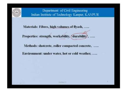
Now, as far as material is concerned, apart from course aggregate, fine aggregate, cement and water. We could use fibers, we could use mineral admixtures. Even if we assume that using mineral admixtures like flyash or blast furnace slag has become common practice either, in the form of blended cements or as additives in concrete itself. There is a special issue involved when we use high volumes of flyash and that is possible and is done in certain specific applications.
