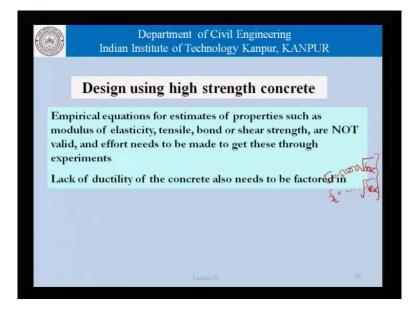
And lastly, coming to some simple things related to design using high strength concretes, we must remember that empirical equations for estimates of properties such as, the modulus of elasticity, the tensile bond or shear strength are not valid and efforts need to be made to get these through experiments.
