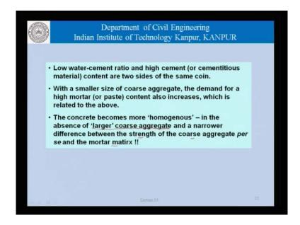
Now, low water cements ratio and high cement or cementitious material content are 2 sides of the same coin. And, we have already talked about that. With a smaller size of coarse aggregates, the demand for high mortar or paste content also increases, which is related to the above that causes us to use more powder in the system. And the concrete becomes more homogenous in the absence of the larger coarse aggregates.
