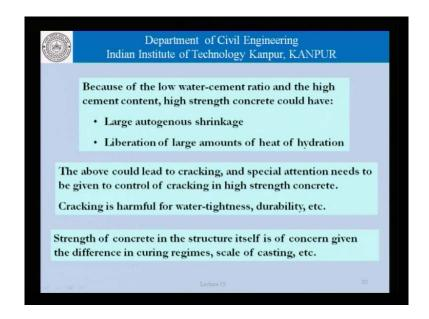
Because of the low water cement ratio and the high cement content, high strength concrete could have large autogenously shrinkage, large amounts of heat liberation on account of heat of hydration. Traditionally, mass concrete was defined as concrete where, the structure was large or the pore volume was large to the extent that the heat dissipation that took place from the surface was not sufficient to handle the heat liberated on account of heat of hydration of cement.
