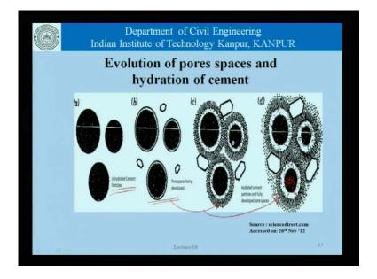
Now, this is another picture of the evolution of pore spaces and hydration of cement. We have unhydrated cement particles suspended in water. Gradually the water in the cement begins to react; hydration products begin to form; we reach a stage like this; and then finally, we reach a stage like this. There is some unhydrated cement which is shown here. And, there are pores spaces within the hydration products, and so on and so forth.
