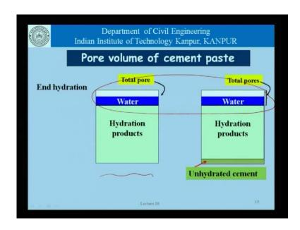
And this is what is the picture; that even at the end of the hydration product, even at the end of the hydration reactions whether it is complete hydration here of the cement or it is unhydrated cement left behind, this part is still true. We still have this space which is available to us, or which becomes available.
