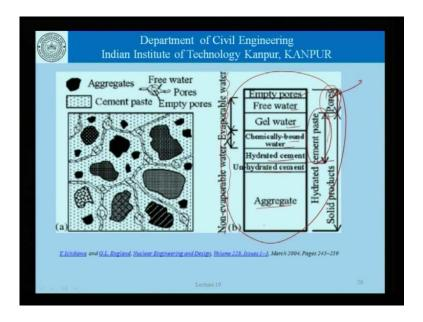
Another model by another researcher is shown here where there are aggregates, there is cement paste, there is free water, there are empty pores, there are saturated pores, and so on. And, this here is some kind of a representation of the different phases- there is aggregate, there is unhydrated cement, there are hydrated cement, there is chemically bound water, there is gel water, free water, empty pores, and so on.
