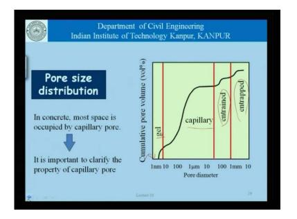
When it comes to entrained air, the size is much smaller; and that is the kind of size that helps us, atleast to some extent in getting more desirable properties. Capillary pores are smaller than that, gel pores are even smaller, and intracrystalite pores are the tiniest of the lot.
