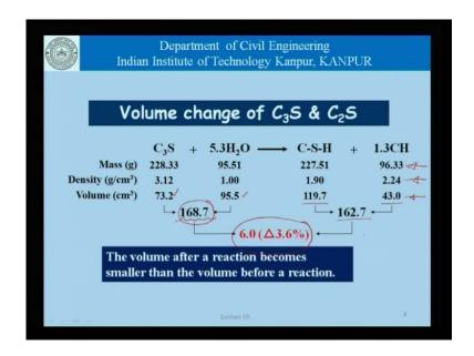
Now, beginning our discussion with the origin of pores and porosity in concrete, let us look at the volume changes that take place when C 3 S and C 2 S which is the tri-calcium silicate and the di-calcium silicate, they hydrate. Now, these equations here give us the chemistry of hydration of these products. As for as C 3 S is concerned, C 3 S plus 5.3 H 2 O gives us C S H which is the calcium silicate hydrate gel, and 1.3 times CH which is calcium hydroxide.
