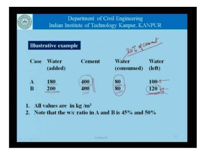
And therefore, the pores will be more, and therefore the strength will be less. Because intrinsically, because strength is related to porosity through an expression which is something like this, which says strength S is equal to S naught times the exponential of minus k times p, where p is the porosity, k is a constant, and S naught is the intrinsic strength of the material. Now, this is something which we will deal with more when we
