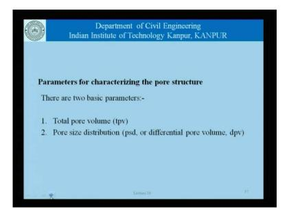
Basically what we use in concrete is 2 parameters to characterize the pore structure- the total pore volume and the pore size distribution, the differential pore volume.
