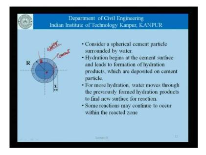
So, having said all that let us take a look at what happens in cement hydration, very quickly. This is a cement particle surrounded by water, and as for as concrete is concerned we can consider millions of cement particles really suspended as for as concrete is concerned in a, in water.
