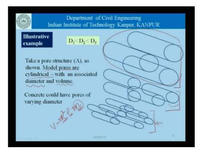
Entrapped air is unintentional air in concrete, entrained air is intentional air through chemical admixtures, capillary pores- they exist within the cement paste and aggregate interfacial zone, the gel pores exist with the gel in the hydration products, and intracrystalites- they exist within the gel.
