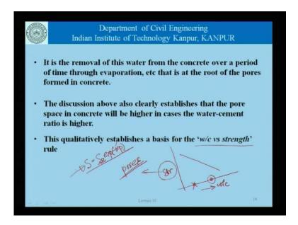
Now, as for as this excess water is concerned which is available in the matrix, what happens to that? It is the removal of this water from the concrete over a period of time through evaporation, and so on, that is at the root of the pores that are formed in
