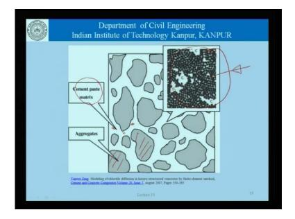
Now, this is a picture of how people try to model these pores and pore structures. These here are large aggregates; they could be sand particles for all you know; it really does not matter. As for as cement matrix or cement paste matrix is concerned the white portion here is all cement paste, and this is what becomes what is shown here in this detail. There are hydration products, and there are pore spaces within the cement matrix.
