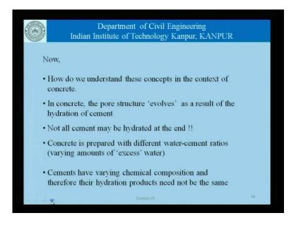
Now, how we do understand these concepts in the context of concrete, where the pore structure evolves as a result of the hydration of the cement, not all cement is hydrated at the end of the day, concrete is prepared with the different water cement ratios which leads to a varying amount of excess water, cements have varying chemical compositions and therefore their hydration products need not be the same.
