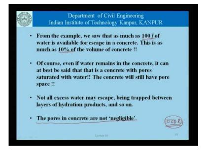
Now, what this example tells us is that as much as the 100 liters of water is available for escape in a concrete containing 180 kgs of water and 400 kgs of cement per cubic meter. And, that is as much as 10 percent of the volume of concrete. We proportion the concrete
