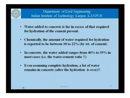
Now, what are the implications of this change in volume as for as concrete is concerned. In addition to the volume changes that take place on account of the hydration of the different phases of cement or different solid complexes of cement. See, C 3 S and C 2 S which we solved just now, are two of the important solid complexes making of the cement. They are the, to be C 3 A and C 4 F, the tri-calcium aluminate and tetra-calcium aluminoferrites.
