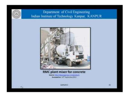
Mixture that is a ready mix concrete plant the concrete is makes for commercial applications, so that is about mixing.
