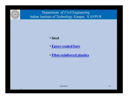
Coming to the reinforcement concrete structures, we know that typically we use steel as a reinforcing material we will not talk much about steel in this course, but we will talk a little bit about epoxy coated bars and fiber reinforced plastics. These two are alternative reinforcing material to steel and are important for a concrete engineer to know because they are answers in cases where concrete is likely to be subjected to reinforcement.
