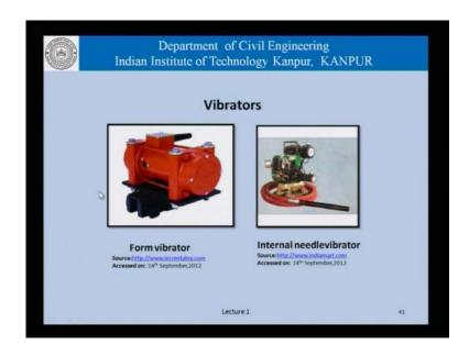
Let us look at vibrations we have form vibrators we have needle vibrators and sometimes we use rural compacted concretes and we have form vibrators which are the stuck or which are applied on the form work and the concrete within is vibrated. We have internal vibrators which is the normal concrete practice with the needle is inserted inside, the concrete that to be placed and the concrete is consolidated into the air and so on, the environment of placing.
