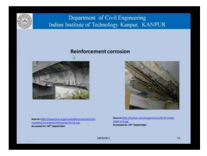
If we look at the pictures here we find that corrosion has caused lot of damage to this concrete structure. It has cause a lot of damage in this part of the structure here we can
