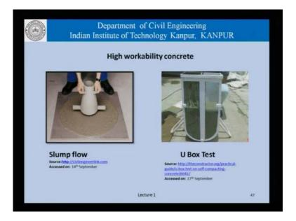
We have shown this picture earlier were this concrete is almost like a fluid it flows. And we use slump flow or the U tube or the U box test to measure its properties under water concrete, we have also seen this picture.
