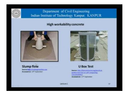
An example of its special properties of concrete, these two pictures here shows high workability concrete and the method that we use evaluate the workability of such concretes cannot be the normal method such as the slump of the compaction factor. There are be the steps like slump flow of the U tube test which is used, we will discuss this later in detail, but we can see that the slum flow here is nothing but how much is the spread of the concrete was the slump cone is removed.
