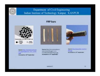
Now, coming to fiber reinforced plastics, now fiber reinforced plastics are F R P bars are basically consist of these fibers, which are embedded in or resin matrix this fibers could be made of carbon or element or glass. There are different materials that can be used for resin and ones this is structure is set then it can be commercially available, and these fiber reinforced plastic bars are available in different shapes and sizes that can we see in this picture here.
