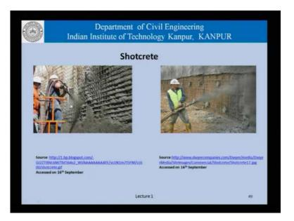
Both of them they referred to shotcrete, shotcreting as you can see here is a process where the concrete is being deposited on the surface without any form work on the other side this makes this concrete very special. We cannot use the kind of concrete here for normal construction, on the other side, if we want to concrete using shotcreters the processs, we cannot use normal materials and process.
