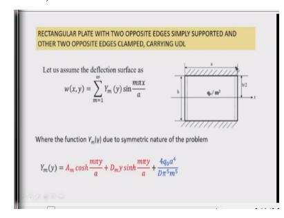
Now, let us see a problem when the rectangular plate a cross b is the dimension, and your thickness is h so that flexural rigidity D is  $\frac{Eh^3}{12(1-v^2)}$ . The plate is loaded with this  $q_0$  is the loading intensity per unit area, and since it is symmetrical, so we pass the axis, x-axis passing through the centre of the edges, which is parallel to y-axis. So, the plate is symmetrical about the x-axis that you can see here.
