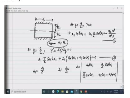
So, since the plate was clamped along 2 other edges, this is clamped condition, this is also clamped. And this  $\frac{a}{2}$  and this is also  $\frac{a}{2}$ , and this is simply supported and this length is also I am taking as a, because it is a square plate. So, imposing the boundary condition at  $y = \frac{a}{2}$ , y = 0, that gives you that  $A_1 cosh$ . If you substitute this  $y = \frac{a}{2}$ , then  $\cosh cosh \frac{\pi}{2}$  will come.
