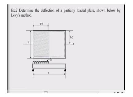
Now, let us discuss another problem of plate which has all the edges simply supported and it is loaded by UDL not up to the full extent of the plate, but up to the middle area. So, it covers only  $\frac{a}{2}$  length of the plate, so plate length is a, and the width is b. Now again, you can note here that the plate is symmetrical about your x-axis. So, therefore I write this equation with the symmetric terms again.
