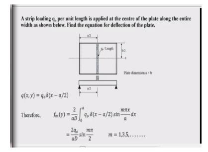
Now, let us consider another problem of plate which has a loading a  $q_0$  per unit length, but in the sense that it is not distributed over the area; it is only a line load that you can call it strip loading. And these loading acts along the y-direction and you can see that this loading is situated at this a by 2, and it is continuous along the y axis. So, that means I can represent this loading with the help of Dirac delta function.
