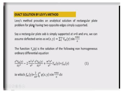
But the difference is that Navier's method the requirement is that all the 4 edges of the rectangular plate should be simply supported. But in case of Levy's method, some relaxation is made. That means only these 2 opposite edges required to be simply supported, and other 2 edges may have any boundary conditions, may have same boundary conditions or may have different boundary conditions or may have elastically supported edge or these supported by torsional spring edge support.
