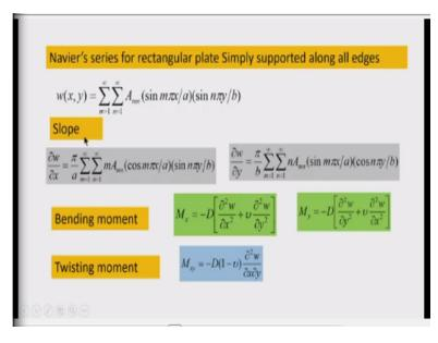
So, other quantities of interest our slope, slope in the x-direction is given by  $\frac{\partial w}{\partial x}$  and it is equal to  $\frac{\partial w}{\partial x} = \frac{\pi}{a}$  summation. And due to differentiation of this sine function this  $\frac{m\pi}{a}$  term will come out. So,  $\frac{\pi}{a}$  is a constant, we have taken outside this summation term and the integer m we have kept inside this summation term. So, it is written like that
