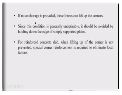
So, if no anchorage is provided, these forces can lift up the corners. Since this condition is generally undesirable, it should be avoided by holding down the edge of a simply supported plate. For reinforced concrete slab, provisions are given in IS code for providing the corner reinforcement to prevent the lifting up of the corner.
