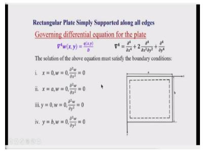
So, let us see the governing differential equation for the plate; the governing differential equation for the plate is given as  $\nabla^4 w(x, y) = \frac{q(x, y)}{D}$  where D is the flexural rigidity of the plate. If the thickness of the plate is uniform, we can assume that D is a constant, and it is given as  $\frac{Eh^3}{12(1-v^2)}$ , where h is the thickness of the plate, E is the modulus of elasticity of the plate material, and mu is the poisson ratio.
