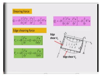
Now, here see these shearing force expressions, shearing force expression is given as this  $\frac{\partial}{\partial x} \nabla^2 w$ ,  $\nabla^2$  is the Laplacian operator. Similarly,  $Q_y$  is also given as  $-D \frac{\partial}{\partial y} \nabla^2 w$ , where,  $\nabla^2$  here is a Laplacian operator. So, it is obvious from these two expressions; edge shear force is also used in
