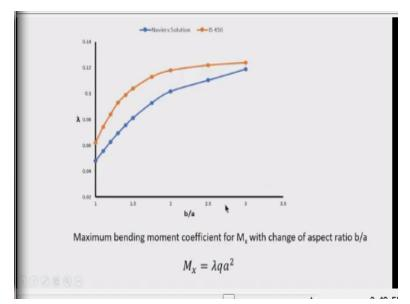
So, if we compute the bending moment, say I take the bending moment along the x-direction with b by a ratio. And we see that our Navier's solution gives a result this with a blue curve that is seen here, that is the variation of bending moment coefficient with the aspect ratio. But if I take the IS code value, because our Indian standard 456 has given the bending moment coefficient for simply supported slab for different aspect ratios.
