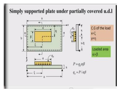
Now let us see a simply supported plate when instead of a fully covered load, a partially covered load is applied. So, again the load is uniform having an area of  $\alpha \times \beta$ , so that is the loaded area. And let us assume that the center of the load is located at the coordinates  $\xi$  and  $\eta$ . So, the
