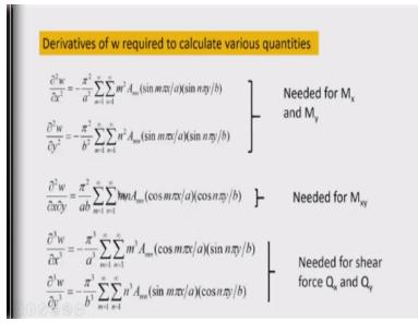
So, for convenience, I was just showing you the other higher derivatives  $\frac{\partial^2 w}{\partial x^2}$  that is  $-\frac{\pi^2}{a^2}$  term will come, and inside this summation, it will be  $m^2 A_{mn}(\sin \sin \frac{m\pi x}{a})(\sin \sin \frac{n\pi y}{b})$ . And it is needed for calculation of M x or M y in both bending moments expression M x, M y these derivatives are needed. So similarly,  $\frac{\partial^2 w}{\partial y^2}$  is given by
