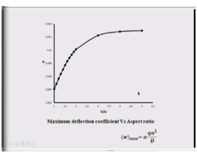
So, if you see the deflection versus aspect ratio curve, you will see that deflection increases with the aspect ratio first and then after it does not increase much and it becomes almost the same, so with the higher aspect ratio.
