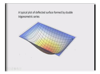
A typical plot of the deflected surface of a simply supported plate looks like that when you superimpose all the waves and if you know the A mn correctly. Then you will get the correct magnitude of the deflection function or deflection surface of the rectangular plate simply supported along all edges subjected to any type of load here.
