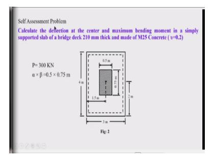
So, I am giving a self-assessment problem just application of this theory partially distributed load and Navier's method. Partially distributed loads are sometimes very useful, especially for bridge deck design. So, the bridge deck consists of full load, and full load may not be fully distributed over the deck slab panel. So, the contact area is distributed only on the tire contact area.
