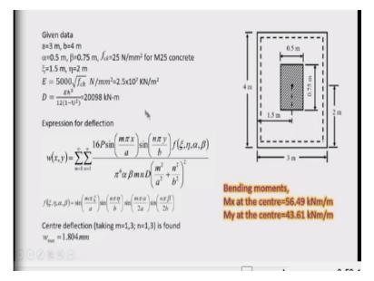
So, the solution is obtained; I am giving some important hints. You can complete and compare the results with the results given here. So, a = 3 meter, b = 4 meter and alpha = 0.5, beta = 0.75, load is placed symmetrically with respect to center. So, our  $\xi$  that is the x coordinate of the center of the load, is 1.5 meter, and y coordinate of the center of the load is 2 meter, modulus of elasticity because in this problem, only this characteristic strength that is grade of concrete is given.
