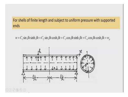
Now, let us apply this theory or solutions that we have written here in the earlier slide for a shell of finite length and subjected to uniform pressure with supported ends. So, here I consider a shell of length l is a closed-cell and it is subjected to inform internal pressure the thickness of the shell is h and the length of the shell is l. So, for convenience, we take the centre of the shell as the origin.
