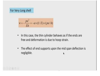
So, for what very long shall we now conclude that  $w = -\frac{pa^2}{Eh}$  and two interesting things we can note here. If the shell is very long and it is a thin shell cylindrical shell, of course, we are dealing with the cylindrical shell behaves as if ends are free and deformation is due to hoop
