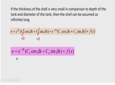
Because the shell is very long. So, as we have treated earlier these two terms have to be dropped otherwise, the deflection and bending moment at the other end will be unbounded. Because this quantity  $e^{\beta x}$  will increase with x because  $\beta$  is a positive quantity. So, therefore, we have to retain only these two constants of integration  $C_3$  and  $C_4$  and the solution now written as  $w = e^{-\beta x} (C_3 \cos \cos \beta x + C_4 \sin \sin \beta x) + f(x)$ .
