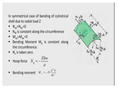
Now, let us see a shell element subjected to load that is radial to the surface normal to the surface. So, I mean that the component of the load along the x-axis and along the y-axis that is the tangential direction to the surface is neglected. So, only loads that are important to cause the stresses in the shell are the load normal to the surface, that is in the radial direction and it is an axisymmetrical type of loading.
