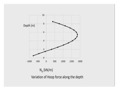
And that variation is plotted here and you can see the maximum Hoop force is obtained here. Say at a distance of these around 5.7 and variation Hoop of force is maximum at this point.
