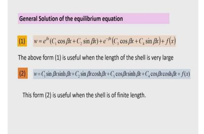
So, general solution of this equilibrium equation differential equation, have been found and it can be expressed in two forms. The one form contains the exponential term and the sinusoidal or cosine functions. So, if I see this form number one that I can see that  $w = e^{\beta x} (C_1 \cos \cos \beta x + C_2 \sin \sin \beta x) + e^{-\beta x} (C_3 \cos \cos \beta x + C_4 \sin \sin \beta x) + f(x)$ . Why it is another function f(x) is added?
