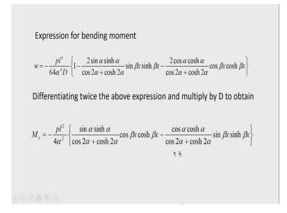
Expression for any moment can be obtained by differentiating the deflection equation two times with respect to x. So, differentiating twice the expression with respect to x, of course, you have to multiply the differentiated quantity with the flexural rigidity of the shell. It is also multiplied with D and finally, we get the bending moment expression.
