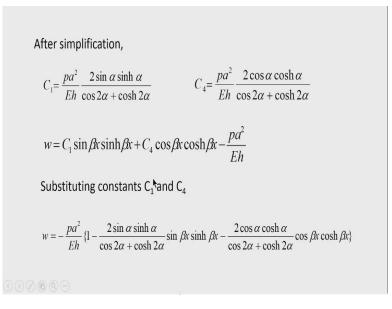
So, using these identities here, we can now express the  $C_1$  and  $C_4$  in simplified form. So,  $C_1$  contains  $C_1 = \frac{pa^2}{Eh} \frac{2\sin \sin \alpha \sinh \sin h \alpha}{\cos \cos 2 \alpha + \cosh \cosh 2 \alpha}$ . Similarly,  $C_4$  contains  $\frac{pa^2}{Eh} \frac{2\cos \cos \alpha \cosh \cosh \alpha}{\cos \cos 2 \alpha + \cosh \cosh 2 \alpha}$ . So, we can now write the complete solution.
