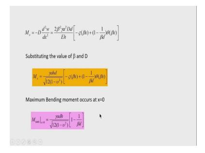
So,  $M_x$  is written after simplification that is putting the value of these various parameters that are appearing here d flexural rigidity that  $\frac{Eh^3}{12(1-v^2)}$  and bringing them in terms of  $\beta$  that is the characteristic parameter of the shell without right the bending moment in the shell as  $\frac{2\beta^2\gamma a^2Dd}{Eh}\left[-\zeta(\beta x) + (1-\frac{1}{\beta d})\theta(\beta x)\right].$
