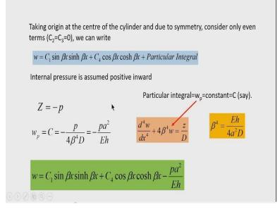
So, with that advantage, we can now reduce the deflection equation with two constants of integration. So, what are the two constants of integration?  $C_1$  and  $C_4$  that were associated with the sin function and sin hyperbolic function and cos function and cos hyperbolic function. So, both are now symmetrical function associated with a particular integral. Internal pressurization positive inward.
