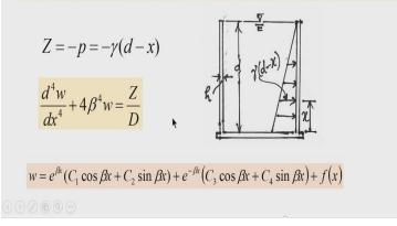
Now, let us apply this solution to another problem that I have told in the beginning of this lecture that a cylindrical shell has to be analysed. And that type of shell is frequently used as water-retaining structure or storage tanks in many applications and the for the solution, we take the wall thickness is uniform, but it is not necessary that wall thickness should be uniform, it may also vary.
