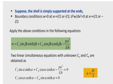
In this problem, we assume that shell is simply supported at the ends. So, boundary conditions now becomes at x = + l/2 or - l/2 say, if x is measured positive towards the right from the origin, then right end support of the shell is denoted by located at x = + l/2, whereas, left-hand support of the shell is located by the distance or coordinate that is x = - l/2.
