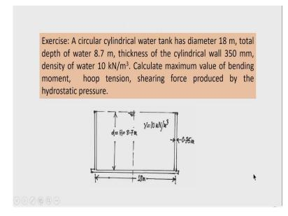
Let us discuss a numerical problem a circular cylindrical water tank has a diameter 18 meter, total depth of the water 8.7 meter, thickness of the cylindrical wall 350 millimetre density of the water 10 kilo Newton per meter cube. We have to calculate the maximum value of the bending moment hoop tension and sharing force, of course, you can calculate produced by hydrostatic pressure.
