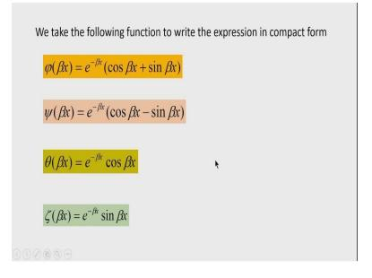
So, these functions are defined as there are several functions which contain this combination of exponential term and cosine and sin term. So, here you can see I have written four functions  $\psi(\beta x) = e^{-\beta x}(\cos \cos \beta x + \sin \sin \beta x),$  $\psi(\beta x) = e^{-\beta x}(\cos \cos \beta x - \sin \sin \beta x),$  etcetera. So, here we abused only these two functions  $\theta(\beta x)$  and  $\zeta(\beta x)$ .
