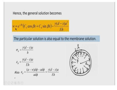
So, now complete solution is written as  $w = e^{-\beta x} \left( C_3 \cos \cos \beta x + C_4 \sin \sin \beta x \right) - \frac{\gamma (d-x)a^2}{Eh}$ . So, this is the particular solution. And again, we will prove that particular solution is also the membrane solution. So, let us prove this, so at any level say x that is defined, x is measured from the bottom of the tank the hoop stress is given by  $\frac{\gamma (d-x)a}{h}$ .
