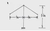
So let us see an exercise for example a conical umbrella roof type roof is to be designed it is made up reinforce concrete and it is supported at the central column. So now let us do this problem take grade of concrete as M20 steel Fe415 and other data for concrete modular ratio is
