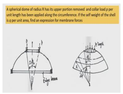
So let us consider one of the, such problem that sometimes a shell having discontinuity means a shell is having an opening at the top. That is sometimes used or a adopted for entry of light and a structure for example a light structure is constructed over this and the load distance is by a edge beam. So this is the edge beam on the shell and this load you can see here I have drawn in a 3D view that load p that is the line load acting along the circumference.
