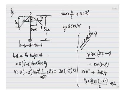
And it is supported on the central column the height of the column is given in the problem as 5.2 meters the base of the cone is 8 meter. The distance from the apex up to free edge of the cone is 1 meter. So the semi cone angle  $\alpha$  is here and  $\alpha$  we can calculate now so given this data we can
