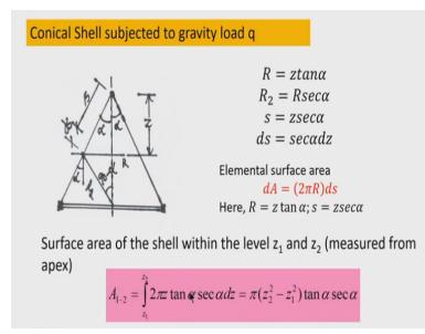
Second problem let us consider a conical shell and we consider there the gravity load that is the vertical load acting on the surface of the shell. Conical shell is also common because this conical
