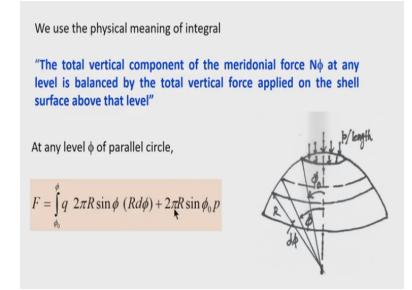
So we use the physical meaning of the intregal says that the total vertical component of the meridional force  $N_{\phi}$  at any level is balanced by the total vertical force applied on the shell surface above that level. So if I consider now a level here so this level is defined from this is the
