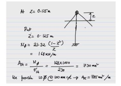
So let us say at say z = 0.125 meter just little away from the apex we calculate this value z = 0.125 meter. That if I see this self-structure z is measured from here and it is the center column this is the center here it is difficult that is at this we have infinite magnitude of membrane stresses especially  $N_{\phi}$ . So therefore let us calculate at distance z = 1 to 5 meter put this z = 1
