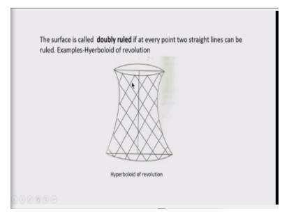
The surface is called doubly ruled, if at every point 2 straight lines can be ruled, examples are a hyperboloid of revolution. For example, this type of shell is specially seen in case of cooling tower. And at every point you can see the 2 straight lines can be ruled. So, 1 straight line is in this direction and 1 straight line in this direction. So, these forms surface which is known as hyperboloid of revolution, so that is doubly ruled surface.
