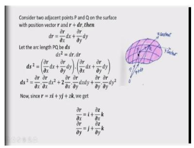
Now, let us see if I can express the dr the small distance from P to Q with the help of the derivative of the position vector then we will be able to find the arc length. So, we can write the vector  $dr = \frac{\partial r}{\partial x} dx + \frac{\partial r}{\partial y} dy$ , where the vector r is differentiated that is the partial differentiation is done here with respect to y and here the vector r is differentiated with respect to x.
