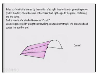
Ruled surface that is formed by the motion of straight lines on its own generating curve is known as directrix. These lines are not necessarily at right angles to the planes containing the end curve. So, there will be 1 end curve, and there will be 2 end curves are there for the shell and the generating straight lines may not be at the right angle. In the previous case we have seen that generating curves are at right angles to the end curves.
