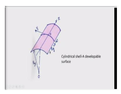
So, cylindrical shell is an example of developable surface.
