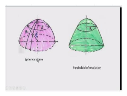
So, that means if I see here, this is 1 example of surface of revolution which is a spherical dome. So, this is the plane curve, it is an arc of a circle and this is rotated about an axis of revolution. Axis of revolution is this and then the surface formed is known as the surface of revolution. So, this is a shell of surface of revolution and it is formed by revolving a part of this circle, the plane curve which is rotating around this axis of revolution is known as meridian.
