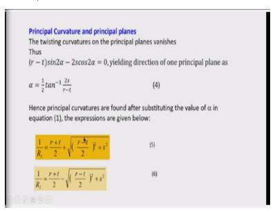
So, based on that twist curvature on the principal planes vanishes and therefore we can write this expression or we can equate this expression to 0. So,  $(r - t)\sin 2\alpha - 2\cos 2\alpha = 0$ , if I make
