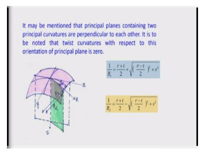
It may be mentioned that principal planes containing 2 principal curvatures are perpendicular to each other. And it is to be noted that twist curvature with respect to this orientation of principal plane will be 0. So, it is clear here if  $\alpha$  is the principal direction, then this plane will contain no
