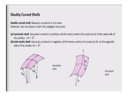
Now let us come to the doubly curved shell. doubly curved shell the Gaussian curvature is non zero. Now if I see the expression of this Gaussian curvature, there is  $rt-s^2$ , that is the result of this product  $1/R_1 \times 1/R_2$ . Now in one case  $rt=s^2$ , that is the Gaussian curvature is 0, we classify the shell as singly curved shell. So, example I have shown that it is a cylindrical shell or it may be a conical shell also.
