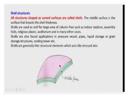
And surface is the main geometrical element or plane; it is the important geometrical element of the shell. Now, all the stresses and that strains etcetera whatever we discuss are referred to the middle plane. So, what is middle plane? Just like our plate middle plane is the plane on middle surface, is a plane which bisects the thickness of the shell, say this is the thickness of the shell and middle plane is bisecting the shell.
