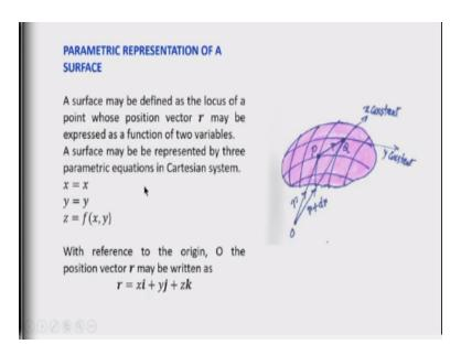
Now as I have told the shell element is characterized by a surface. So, let us see what are the fundamental properties of the surface? And how the surface can be represented with the parametric equations? So, here you can see a surface and the curved lines you are seeing in both direction orthogonal direction in x direction as well as in y direction. Suppose this is one direction that is aligned along the x axis.
