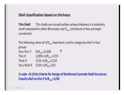
Now some authors prefer the shell classification based on thickness, but the shell classification based on geometry is mainly on curvature. Shell classification based on curvature is mainly recognized. Based on thickness, the shell is classified into 4 categories, very thin, thin, thick and very thick. Now how the categories are found? These categories are found based on this thickness to this minimum of the 2 principal curvatures.
