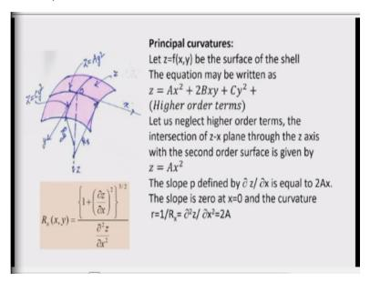
Based on that, now let us define the principal curvatures. The principal curvatures will be useful to classify the shell. Now let z=f(x,y) be the equation of the surface of the shell or the equation of the shell. Actually we will not call this as a plane because it is a curved structure, so therefore it is called as a surface and this is a curved surface. So, z=f(x,y) if it is expressed in the polynomial form, say generally it is a curve, so it will be a nonlinear function.
