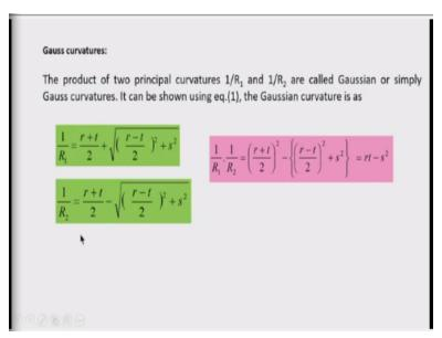
Now let us define a term based on the principal curvature applicable to the shell surface. If I see that  $^{1/R_{1}}$  is a principal curvature and  $^{1/R_{2}}$  as another principal curvature and get the product of the 2 principal curvatures which is called as Gaussian curvature or simply Gauss curvature. So, if
