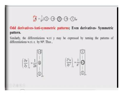
So, after adding, we get the 1st term is 1, 2nd term is -4, 3rd term is 6 then 4th term is -4 and 1. So, you can see here that this the 4th derivative in the molecular form is written, the central value is 6, coefficient of deflection in the nodal point there is the node centering which you will write the finite difference equation that coefficient is 6. And towards right and towards left, the same coefficient appears because it is even number of derivative, so the quantities are symmetry.
