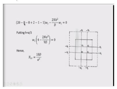
So, after simplification, now we can write this and putting 20 - 8 - 8 + 2 - 1 - 1. And this is, if you simplify it, it will be  $-2w_1$ , so, therefore, it is  $-\frac{2w_1Nh^2}{D}$  by putting h = a/3 because we have divided the plate into 3 equal parts. We now write  $w_1\left(4 - \frac{2Na^2}{9D}\right) = 0$
