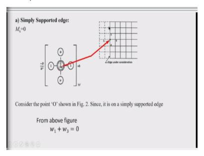
We consider a simply supported edge; this edge is simply supported. So, this is the plate domain that is shown by solid lines. But dotted lines are not really existing it is taken for this finding the expression in terms of the displacement of the plate domain. Now let us say this edge M = 0, so our stencil was this for this bending moment. So, if I put this is the node, so if I put this here, just I take this here.
