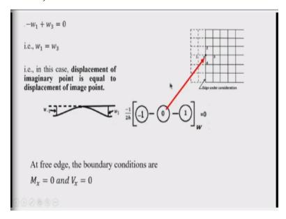
So, now this stencil is now put here; 0 is the node where you want to apply the boundary conditions. So, this fixed that is the slope this stencil is first derivative stencil is put here at 0. And then we get that 2 points; this point is on the node on the boundary. This point is on the boundary, so therefore automatically, it vanished because the deflection at the boundary is 0. But this node is outside the boundary and with coefficient -1.
