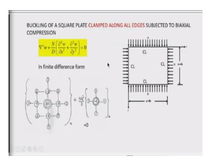
Now, here again, I give you one problem that you can see it is solved in a similar way, but the edge condition is now altered. So, edge condition is now clamped instead of simply supported, and this is the stencil for the plate buckling equation.
