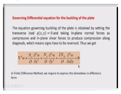
Now, let us see the differential equation. As you know that differential equation of the plate subjected to the axial compression  $N_x$  and  $N_y$ . And the in plane shear  $N_{xy}$  given by this equation
