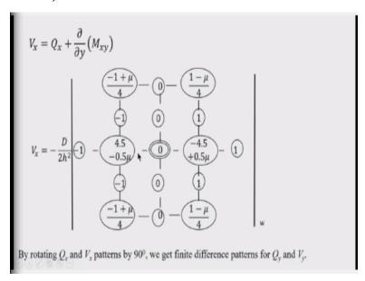
So, therefore  $V_x$  that is along the x = a or some edge at the boundary, you want to apply the edge shear condition as a boundary condition. Another boundary condition at the edge is say bending moment, specially for free edge the boundary condition becomes if x = a edge is free, then the boundary condition at x = a will be $M_x = 0$  and  $V_x = 0$  So, instead of 3 equations that we earlier told that  $M_x = 0$ ,  $Q_x = 0$  and  $V_x$  and  $M_{xy} = 0$ .
