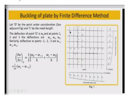
Say a domain of the plate, here it is shown, and this is divided into several divisions, and for simplicity, I am taking the equal size of the mesh in both direction x and y, but it may be
