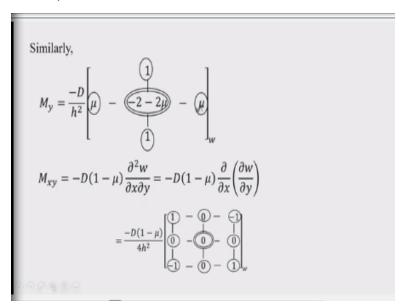
So,  $M_y$  is written like that you can see the difference, this is just placed now in the horizontal position, this vertical is now placed in the horizontal position, so we get this the  $M_y$ , so  $M_y$  is obtained like that. Then  $M_{xy}$  the mixed derivative is also needed because if we consider the shear buckling, how the shear buckling equation is formed? Shear buckling equation is formed with the term  $\frac{2N_{xy}}{D} \frac{\partial^2 w}{\partial x \partial y}$ .
