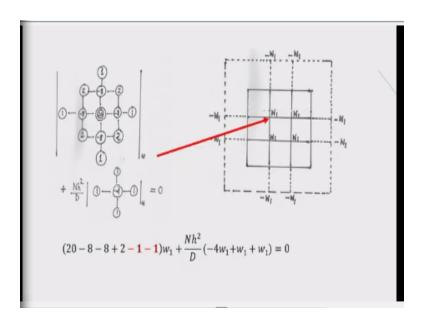
So, now place this stencil. So, this is the stencil for the buckling equation of the plate; that is, you can tell it the molecular form. So, if we now place the stencil here, there are 2 parts one is for plate bending that you can see,  $\nabla^4 w$ , and this is for buckling part, that is  $\frac{Nh^2}{D}$ . So, now let us first place this, if I place this here, then  $20w_1$ , so  $20w_1$  is coming. Then here this circle is falling here, so -8.
