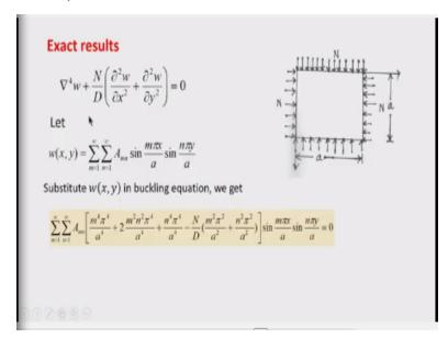
So, if I see the differential equation is this, and the edge condition is simply supported. Then I can take the double trigonometrical series that Navier series to find the solution of the deflection. That is, I want to solve it by exact method. So, therefore substituting this in the differential equation.
