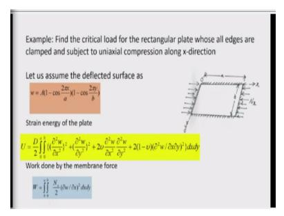
Let us illustrate this method with an example. So, I have taken an example of this plate which has this fixed edges, so all the edges are fixed. So, this type of problem cannot be solved by using the Navier's method or the Levy's method. So, therefore we take the help of approximate method. Now here you can see the assumed deflection function, I have taken only the first term other terms can also be written taking origin at O.
