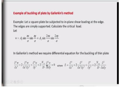
Now we take the function, the shape function as consisting of 2 terms of the Navier series. Because we have taken the support as a simply supported, so we take the support as simply supported and therefore we take this shape function as consisting of the 2 terms of the Navier
