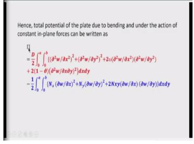
So, now with the help of this we can now write the total potential capital  $\Pi$ . So, total potential capital  $\Pi$  for the buckling problem is now given as D/2 integration 0 to a, 0 to b that is the curvature in the x direction square + curvature in the y direction square +  $2 \times v$ , y is the Poisson
