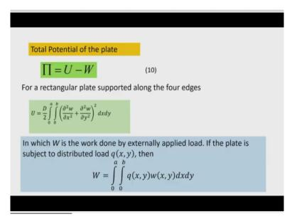
So, knowing the strain energy expression for the plate or any structural element whether it is beam or other elements then we can find the total potential of the system. Here I am mentioning plate because the course is focused on the plate only, but this term that I have written  $\Pi = U - W$  can be used for any type of structural element also. So,  $\Pi$  is the symbol that is used here to denote the total potential of the plate.
