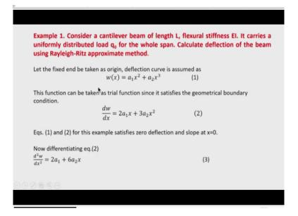
So, let us see an example, first consider a cantilever beam of length L, flexural rigidity EI, I have selected a problem of beams, so that you can understand the concept of this problem and then you can apply to the plate problem. So, it carries a uniformly distributed load  $q_0$  for the whole span. Now we required to find the deflection of the beam using Rayleigh-Ritz method.
