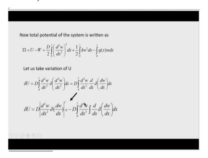
Now we write the total potential  $\Pi$  equal to U - W. So,  $(U = \frac{D}{2} \int_{0}^{l} \left(\frac{d^2 w}{dx^2}\right)^2 dx) - W$ , and what
