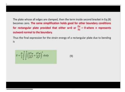
Now, we can see that some plate has edges which are clamped, there are many plates which all edges are clamped, it is argued like that the plate whose all edges are claimed then the term inside the second bracket in equation 8, actually the second term the term inside the second bracket, this is the term inside the second bracket can be ignored or it vanishes.
