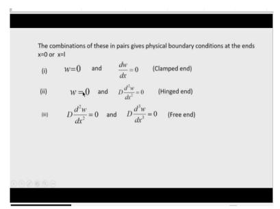
The combinations of these in pairs give the physical boundary conditions at the ends, x = 0and x is = 1. So, x = 0. Now, one combination is w = 0,  $\frac{dw}{dx} = 0$ . So, that combination gives clamped end, and another combination may be w = 0,  $D\frac{d^2w}{dx^2} = 0$ . This combination gives his hinged end or pined end, or simply supported end. Then the third combination, the  $D\frac{d^2w}{dx^2} = 0$  and  $D\frac{d^3w}{dx^3} = 0$ .
