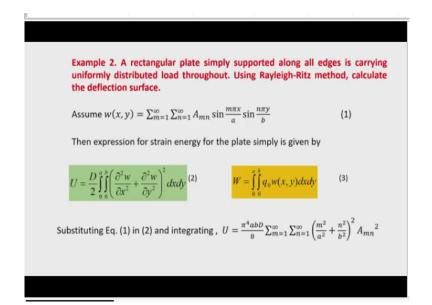
Now we give you a plate problem example. So, take a simply supported plate which conveniently expressed, deflection is explained by the double trigonometrical series because you know that  $\sin \sin \frac{m\pi x}{a} \sin \sin \frac{n\pi y}{b}$ . If these terms are summed up, up to infinite series, then it represents the deflection of a simply supported plate. That means the plate is having all edges are simply supported.
