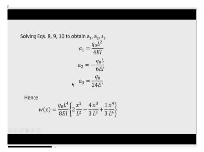
We now obtain  $a_1$ ,  $a_2$ ,  $a_3$ . So, obtaining this  $a_1$ ,  $a_2$ ,  $a_3$ , we now express the deflection. So, from this deflection equation, we can now obtain the slope, bending moment and shear force using the derivative of the deflection function.
