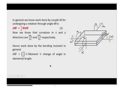
Now, let us see in general, we know that work done by the couple M. M is any couple for undergoing a rotation to an angle  $\theta$ . You can see that the strain energy is nothing but by the work done by the external force, which is stored as a strain energy. So, in that case, suppose a body is deformed by a force; here, of course, the body is undergoing the rotation due to application of bending moment.
