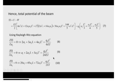
And then, the total potential is obtained and using Rayleigh-Ritz equation because here 3 constants are involved, 3 terms are used in expressing the deflection. So, we use the partial derivative of  $\frac{\partial \Pi}{\partial a_1}$ . Again,  $\frac{\partial \Pi}{\partial a_2}$  and  $\frac{\partial \Pi}{\partial a_3}$  and these 3 partial derivatives are evaluated and equated to 0. So, we get 3 linear equations involving  $a_1$ ,  $a_2$ ,  $a_3$ .
