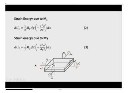
So, knowing this fact now, we can write the strain energy due to  $M_x$  is  $dU_1$ , say this part is  $U_1$ , contribution towards the strain energy due to bending moment along the x-axis is  $U_1$ . So,  $dU_1$ , we can write  $\frac{1}{2}M_x dy$ , why it is  $M_x dy$  because  $M_x$  is acting along the edge whose length is dy. So, therefore,  $M_x dy$  is the total bending moment along this edge because  $M_x$ ,  $M_y$ , etcetera are considered to be quantity per unit length.
