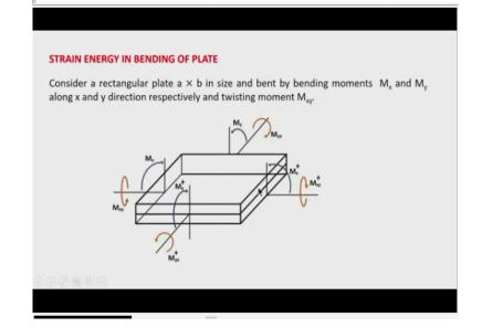
Now, let us see strain energy expression for the bending of plate. So, here you are seeing that a plate which is a dimension A, B and in that case, we take an element of the plate whose length is dx along the x-direction and dy along the y-direction. So, moment you are seeing  $M_x$  is the bending moment along the x-axis, and on the opposite side, the  $M_x^+ M_x^+$  increment of the moment is  $\frac{\partial M_x}{\partial x} dx$  along the x-direction.
