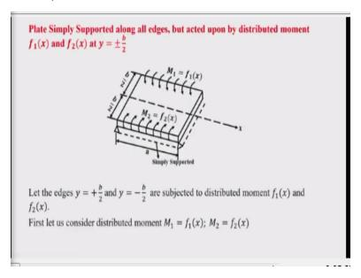
So, now let us consider a plate, rectangular plate, length is a and width is b subjected to distributed moment along the edge y = 0, the moment is  $M_1$  which is distributed along the x axis in a functional form that I have written  $f_1(x)$ , this may be a constant also or may have any other variation. Then on the opposite edge y = b, here you will see that the moment  $M_2$  is acting and which is in the functional form is expressed as  $f_2(x)$ ,  $f_2$  is a function of x.
