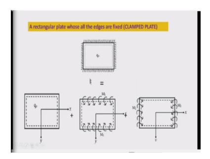
Now let us see the second case, that is the most important condition in practical purpose, the all edges are fixed in most of the cases for better rigidity and for better stability of the structure. So, here you can see that because of the clamped condition along 2 edges neither Navier condition nor Levy's condition will yield the closed form expression. So, this is decomposed into 3 parts that we need to superimpose.
