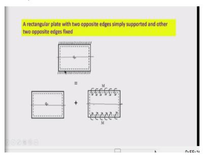
Let us see in the first case, we have to deal with this condition, that of course already obtained in my earlier classes, that 2 edges are simply supported x = 0 and x = a are simply supported, if this length is a and this is b. And this is clamped y = 0 and y = b is clamped, but of course here we are taking the x axis running through the middle of the plate. So, naturally the boundary condition will specify at y = +b/2 and y = -b/2.
