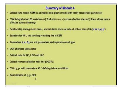
So, it is a summary of module 4. Critical state model CSM is a simple elastoplastic model with easily measurable parameters. Now there are several other models as well, but what makes it different is that it is simple to understand. And the parameters are easily measurable from whatever routine tests that we know, so that makes it a bit different from the other models. CSM integrates two 2D variations, the void ratio versus effective stress and shear stress versus effective stress.
