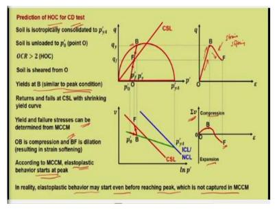
So, now let us see prediction of HOC for CD test. Soil is isotropically consolidated  $p'_{yA}$  and it is unloaded to  $p_o'$ , the same procedure. But then now the unloading is a bit more, so that HOC state gets emerged and OCR is greater than 2, so that we already know. So, again the repetition of the same, now only thing is here it is volume change and we need to consider both compression and expansion.
