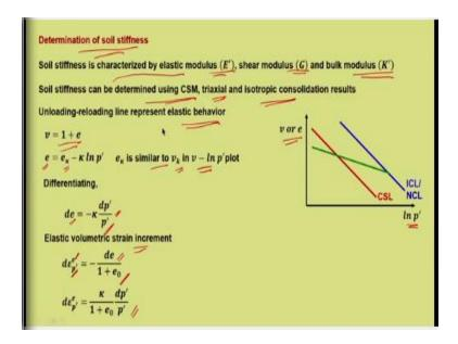
Now that is all related to the prediction and another aspect that we can predict based on critical state framework or very specifically MCCM is the soil stiffness. So, the next discussion is determination of soil stiffness. Soil stiffness is characterized by elastic modulus E', shear modulus G and bulk modulus K'. K' and E' is shown to show that this is relevant only for effective stress condition when it comes to soil behaviour.
