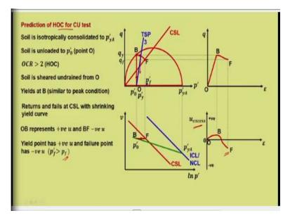
Now for CU test for HOC. So, we have defined all the four combinations that is NC LOC, CU CD, HOC CU CD. So, now we will discuss CU test. Soil is isotropically consolidated to  $p'_{yA}$ , again the same condition let us skip this, it is the same condition. So, u excess, now instead of cumulative volume change, now we have excess, excess pore water pressure. Same yield curve, everything remains same, loading, unloading curve,  $p'_o$  the point O, the initial point critical state line.
