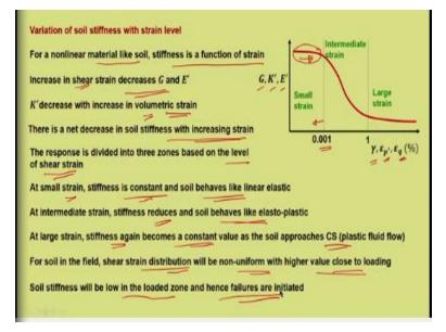
A variation of soil stiffness with strain level, we can note that for a nonlinear material like soil stiffness is a function of strain, it keeps changing. So, at a low strain we know it is a linear response and then it becomes a nonlinear response. Now increase in shear strain decreases G and E'. K' decreases with increase in volumetric strain, because each of this is associated with shear response and volumetric change.
