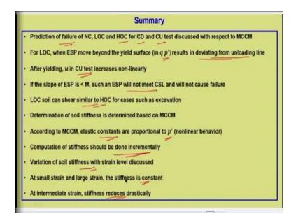
So, that is all about a prediction based on MCCM. Let us summarize today's lecture prediction of failure of NC, LOC and HOC for CD and CU test discussed with respect to MCCM. For LOC, when ESP move beyond the yield surface that is in q p' plot, it results in deviating from the unloading line. So, we have shown that relationship with respect to yielding and the yield curve. So, from unloading reloading line it deviates towards the critical state line.
