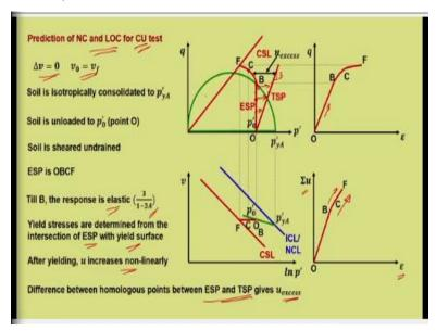
Now prediction of normally consolidated LOC for CU test, now initially it was CD test, now it is CU test, most of the discussions remain same only thing is the volume change is replaced by excess pore pressure generation. And this is again a prominent point we know, there is no volume change so  $\Delta v = 0$   $v_o = v_f$  so this is a very important clue for solving the problem.
