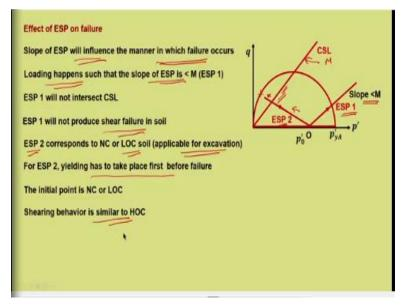
So, effect of that is all about heavily over consolidated and the prediction of  $q_f$ ,  $p'_f$ ,  $q_l$ ,  $p_y$  will happen based on the geometry of the figure and by substituting the relevant equations in combination with the yield curve. So, we will come to that when we solve the problem. So, effect of ESP on failure. So, we just need to understand 2 important points here, slope of ESP like in what manner it is loaded.
