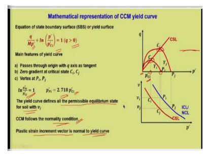
So, we have understood the basic framework and now the equation of state boundary surface or yield surface, that is how do we represent this particular yield curve. The logarithmic spiral yield curve is given by this expression which is
