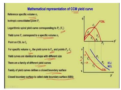
So, let us understand what is the mathematical representation of Cam Clay model yield curve. Let us consider a specific volume of  $v_i$ , so this is q p' plot and this is vp' plot. Now let us consider the reference  $v_i$ , so this is the  $v_i$  corresponding to which there is an initial consolidation point which is  $P_i$  on the ICL, NCL. Now this can be either isotropically or it is one dimensional consolidated point  $P_i$  for which the specific volume is  $v_i$ .
