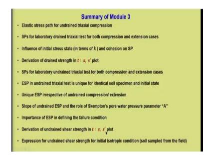
Elastic stress path for undrained triaxial compression, we have already seen that. Stress path for laboratory drained triaxial test for both compression and extension, we have discussed all the 4 cases with different permutation, combination. Influence of initial stress state that is in terms of k value and what is the influence of cohesion on the stress path, we have seen that it gets extended above, so the available strength increases.
