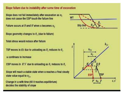
Now, if the slope fails after some time of excavation, so, what will happen? Slope does not fail immediately after excavation as  $u_i$  does not cause the ESP to test the failure line. So, this case is different, but the failure happens after some time of excavation. So, the initial
