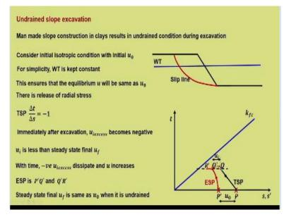
Now, let us deal with un-drained slope excavation. Manmade slope construction in place results in un-drained condition during excavation. So, here also we are dealing with slope but a finite slope instead of an in finites. Now, this is a given finite slope, this has been created because it got excavated from this end. So, consider initial isotropic condition with initial  $u_0$ . For simplicity, water table is kept constant and why we want to maintain this?
