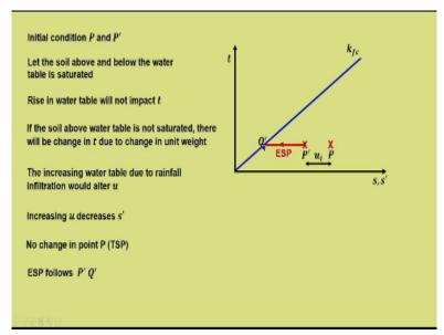
So, initial condition P, P', so, let us try to plot these conditions on t-s, s' plot. So, let us say P is the initial condition and there is an initial pore water pressure of u<sub>i</sub>. So, this difference will be u<sub>i</sub>, so, P and P' is separated by u<sub>i</sub>. Let the soil above and below the water table is saturated. Let us presume that it is because of capillary rise or whatever the soil sample above the water table is also saturated.
