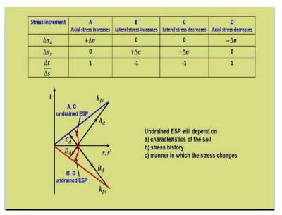
So, let us try to understand this on t-s, s' plot. This t-s, s' plot and let the starting point be same, let us assume. So, the first stress path that is corresponding to case A is typical drained stress path. So, let us first talk about drained stress path and those that an inclination of 45 degrees and  $A_d$  the presence the case A. Now, case B that is lateral stress increase. It is towards extension now, when the stress path moves towards the blue line, that means it fails in compression.
