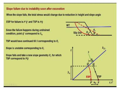
Now, slow failure due to instability soon after excavation. So, when the slow fails, the total stress would change due to reduction in height and slope angle. So, what is happening? When there is instability, there is a failure which happens to this slope and because of this failure,
