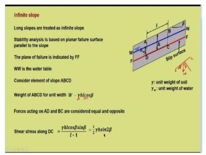
So, let us first take the case of infinite slope. And what is an infinite slope? Long slopes that are treated which are long are treated as infinite slope. For example, a mountain and the planar area gets extended over a long distance. That can be treated as an infinite slope. Whereas the smaller slopes for example in the case of embankment, these are finite slope. So in long, huge hills and big mountains, the slope can be treated as planar and it can be treated as infinite slope.
