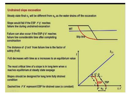
Now, we will see 2 different cases that is steady state final  $u_f$  will be different from  $u_0$  as the water drains off the excavation. So, in the previous slide, we have assumed that there is no change, but now if it starts draining off, then the final pore water pressure  $u_f$  will not be same as that of the initial pore water pressure  $u_0$ . Slope would fail if the ESP that is P'Q' reaches failure during un-drained excavation.
