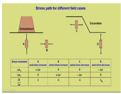
So, let us first take the case of an embankment. So, here, it is a manmade embankment and hence, what is the consequence of the construction of this embankment is that the stress acting on the soil increases. So, immediately below the embankment, if we consider a cylindrical soil mass, then what happens is because of this embankment there is an increase in the stress acting on this.
