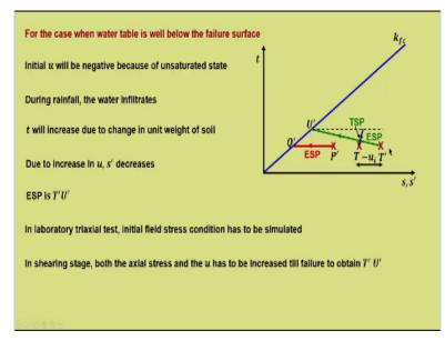
For the case when water table is well below the failure surface, now, we have considered the case where water table is above the failure surface. Now, here let us try to see what difference will it make from P'Q', if the water table is well below the failure surface. Now, what is the implication when water table is below? When the water table is below, the pore water pressure in the along the failure surface will be initially negative.
