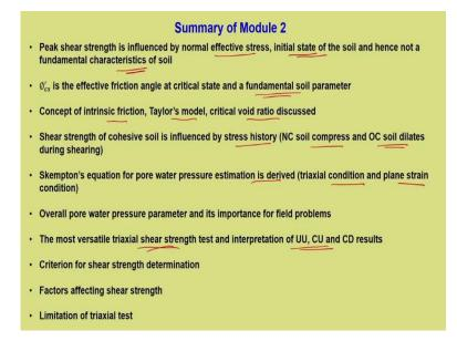
Now, peak shear strength is influenced by 2 important aspects. One is the normal effective stress and the other one is initial state of the soil. Now, when I say normal effective stress that confinement restricts the dilation and when I say initial state it has something to do with how
