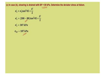
In the case 3, shearing is done but there is a back pressure of 80 kPa. So, what will be the deviatoric stress? Same procedure, only thing is here  $\sigma_3$ ' changes. You need to find out what is  $\sigma_3$ '. And  $\sigma_1' = 307 \ kPa$  and  $\sigma_{df} = 187 \ kPa$ .
