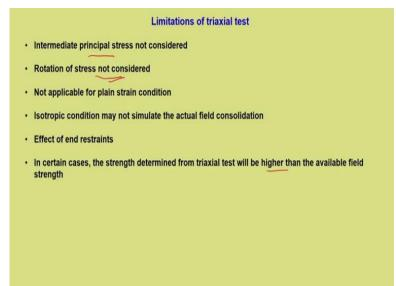
So, that is all related to what are the factors affecting the shear strength. Next is limitations of triaxial test. In triaxial test, we do not consider the effect of intermediate principal stress quite obvious. Rotation of stress is not considered which is a common phenomenon. If you consider the slope and the slip line you can see that the principal stress rotation happens. Now, this is not considered in triaxial testing rather it is not possible.
