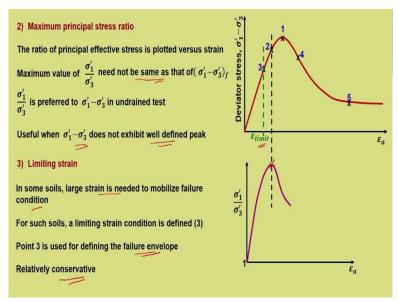
Now, the maximum principal stress ratio, a very useful way of representing stress strain behavior and obtaining the failure envelope for especially for un-drained case. The ratio of principle effective stress is plotted versus strain. You have seen this in the previous slide. Maximum value of  $\sigma_1$ '/ $\sigma_3$ ' need to be same as need not be same as that of ( $\sigma_1$ '- $\sigma_3$ ')<sub>f</sub>.
