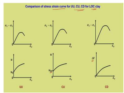
So, we will see the first aspect is the comparison of stress strain curve when you have all the 3 tests done on a particular soil. All the other conditions remaining same, how will these results compare, I mean to say UU, CU and CD. This comparison is not conclusive but a conceptual comparison we can say. So, the first one is UU test, the stress strain response and the pore water pressure generation as u nought is the initial pore water pressure before shearing.
