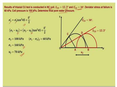
With that we finish the discussion and the additional aspects. We will just see a very small brief problems just to make sure that what is the influence of pore water pressure on the shear strength. So, the first problem is results of triaxial CU test is conducted in NC soil.  $\Phi_{CU} = 13.3$
