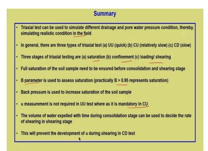
So, the triaxial test can be used to simulate different drainage and pore pressure condition thereby simulating realistic condition in the field. In general there are 3 types of triaxial test UU, CU and CD. There are 3 stages that is required in the triaxial testing which is the saturation, confinement and loading or shearing. Full saturation of the soil sample need to be ensured before consolidation and shearing stage.
