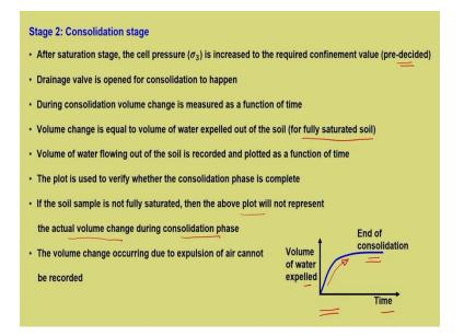
Stage 2 is the consolidation stage after saturation stage the cell pressure is increased to the required confinement value which is already pre decided by the person who is conducting the test the drainage valve is opened for consolidation to happen. Now none of this was relevant in UU test,
