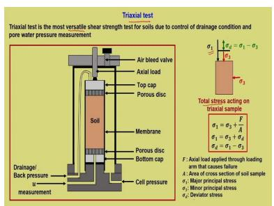
So, this is all about triaixal test. So, triaxial test is the most versatile shear strength test for soils due to control of drainage condition and pore water pressure measurement. Now in the field you have different possibilities a low permeable soil has the drainage capacity quite low which means
