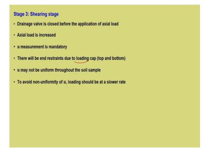
So, next is the shearing stage of CU test where drainage valve is close before the application of axial load and then axial load is increased which is the deviator load, u measurement is mandatory we have seen they will be end restraints due to loading cap whatever this particular aspect we have already discussed u may not be uniform throughout the soil sample to avoid the non uniformity of u loading should be at a slower rate.
