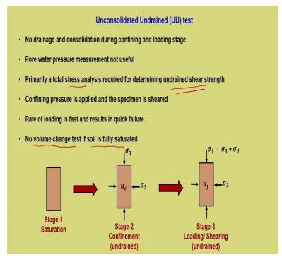
So, let us see the features of unconsolidated undrained test we are not going to discuss any results in this lecture we will understand clearly what are the possibilities of these tests, no drainage and consolidation during confining and loading states we have seen this now pore water pressure measurement is not useful. This is an undrained test what else is going to happen other than pore water pressure. But still one can always measure the pore water pressure in UU test.
