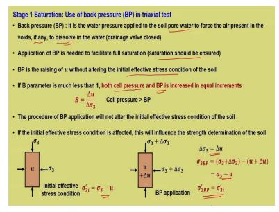
As I told in the beginning we will discuss a bit on what is back pressure in triaxial testing and this backpressure is applicable for all the 3 testing because back pressure is useful for saturation and saturation is mandatory for all the 3 types of tests, all the 3 types of triaxial testing. Now what is back pressure? It is the water pressure applied to the soil pore water. So, it this pressure goes within the soil sample to force the air present in the voids if any.
