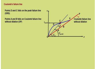
So, Coulomb's failure line; how these ABCD translates to columns failure line, this is the critical straight line fi dash cs and depending upon the amount of dilation, there will be a kind of peak angle which gets added is a dilation angle which gets added to fi dash critical state and that results in fi dash peak. So, we can see that C and D falls on the big failure line. So, it also depends on the kind of confinement it has.
