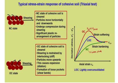
So, typical stress-strain response of cohesive soil: Now, more or less things remain same the y axis, x axis have changed, but the response remains more or less similar. For an NC soil that is NC, state when it is sheared, we can see that it is a loose state, why it is a loose state, because it has not been stressed too much in the past. So, NC, state of cohesive soil is sheared particles move horizontally and downwards because it is in a loose state undergo compression during shearing.
