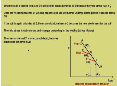
So, when the soil is loaded from C to D, it will exhibit elastic behaviour till D because the yield stress is at  $\sigma'_B$ . So that is an important aspect which is very important for module 4. So, up to  $\sigma'_B$  since the yielding has not occurred, so, up to  $\sigma'_B$  it will exhibit and kind of elastic
