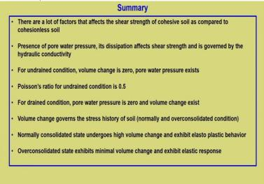
To summarize, there are a lot of factors that affects the shear strength of cohesive soil as compared to cohesionless soil. Presence of pore water pressure its dissipation effects shear strength and are governed by its soil hydraulic conductivity. For undrained condition volume changes 0 and pore water pressure excess. Poisson's ratio for undrained conditions 0.5 for drain condition pore the pressure is 0 and volume change exists.
