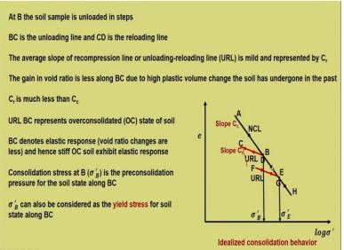
So, this much we need to keep in mind. So, a normally consolidated soil undergoes elastoplastic response. Now, let us say that at B the soil is unloaded and it is unloaded in steps BC is the unloading line and CD is the reloading line. So, it is an unloading reloading line the slope of this unloading reloading line or it is called recompression line it is mild and it is represented by Cr.
