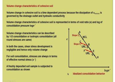
So, volume change characteristics needs some more discussion let us see, volume change in cohesive soil is a time dependent process because dissipation of u excess is governed by drainage outlet and hydraulic conductivity. Volume change, characteristics of cohesive soil is represented in terms of void ratio and log of consolidation pressure which is the net result of consolidation test.
