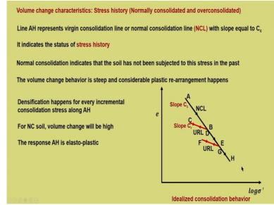
So, in this line AH is known as virgin consolidation line or normal consolidation line, NCL and it have got a slope of  $C_c$  which is which is known as compressibility index. Now, why this is called virgin consolidation line I hope you would have understood during your UG because any stress on this AH it is for the first time the soil is experiencing that is the reason why it is called virgin consolidation line and very popularly known as normal consolidation line.
