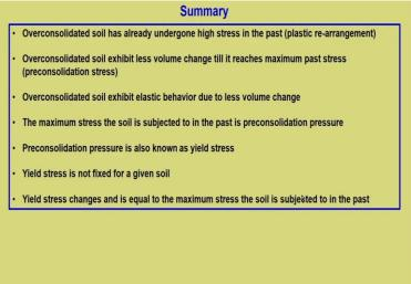
Over consolidated soil has already undergone high stress in the past which is plastic rearrangement. So, over consolidated soil exhibit less volume change till it reaches the maximum past stress which is the preconsolidation stress. Over consolidated soil exhibit elastic behaviour due to less volume change. The maximum stress the soil is subjected to in the past is called preconsolidation pressure.
