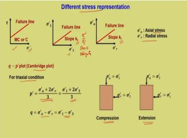
So the first one is about different stress representation, the first one is familiar to us which is  $\tau$  versus  $\sigma$ ' where  $\sigma$ ' is the effective normal stress. Now you need to note a specific point here, I have started introducing dash or prime. Now this is very important because now, we have started the actual discussion of strength and we know by effective stress principle strength is completely governed by the effective stress.
