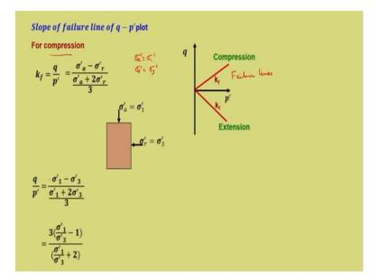
Now, let us see the slope of the failure line in q-p'plot. So what is the slope of  $\tau$  versus  $\sigma$  plot? It is nothing but  $\phi$ ', so that is the slope. Similarly we want to find out what is the slope of failure of q-p'plot. So this is q-p'plot and I have drawn 2 lines, these are failure lines and one line corresponds to the case of compression, the other line corresponds to the case of extension.
