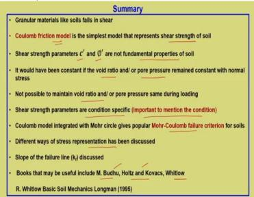
So that is all about that. So we will summarize this first lecture that is granular materials like soils fails in shear. We have already told this we need to keep this in mind. Coulomb friction model is the simplest model that represents shear strength of soil but remember Coulomb friction model, it depends upon the development of a failure plane within the soil mass. Shear strength parameters c' and  $\varphi$ ', these are not fundamental properties of soil.
