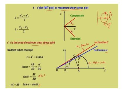
Now another representation of stress is t -s' plot or it is called MIT plot or it is known as Maximum Shear Stress plot. What is maximum shear stress? When you draw a Mohr circle, we know that there is a maximum point that we obtain and we have seen that this maximum point is not the stress which causes failure but a critical combination causes failure. So here we will specifically talk about the maximum shear stress point.
