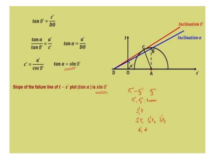
Now we also note  $\tan \varphi' = c' / DO$  that is  $\tan \varphi'$ , considering the red line, the intercept is c' divided by DO. If I write  $\tan \alpha / \tan \varphi'$  where  $\tan \alpha = a' / DO$ , we can write a' / c'. So  $\tan \alpha / \tan \varphi' = a' / c'$  from which we can write, how will we get this? So  $\tan \varphi'$ , we have already seen  $\tan \varphi' = \sin \varphi'$ , we have already proved. Substituting that here in this expression  $\tan \alpha = \sin \varphi'$ .
