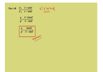
Now, we have  $\sigma'_1 = \sigma'_3 \tan^2 (45 + \varphi'/2)$  this is as per the Mohr Coulomb failure envelope. Now this is not going to change, this remains same. So we have what is the ratio? Now this is for c' = 0, we are not considering cohesion for the time being, so we will consider the Mohr Coulomb failure envelope that will give  $\sigma'_1 / \sigma'_3 = \tan^2 (45 + \varphi'/2) = 1 + \sin \varphi'/1 - \sin \varphi'$ .
