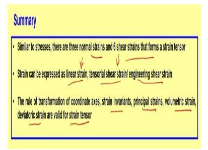
So to summarize the strain acting in the soil, similar to stresses there are 3 normal strains and 6 shear strains that form a strain tensor. It can be expressed as linear strain or it has a tensile strain engineering shear strain. So, one is normal component and the other one is shear component of strain which is tensorial shear strain or it is known as engineering shear strain. The rule of transformation of coordinate axes we have discussed for stresses.
