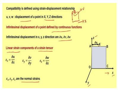
Now, compatibility is defined using strain displacement relationship. Now, we can say that u, v, w these are displacement of a point in x, y, x direction okay. So u, v, w for example if I have a body like this and I am discussing about this point. This point may undergo, it is a microscopic phenomenon, I am just analyzing it and showing you, so this change this displacement if this is an x direction, then this corresponds to u, so that is what it means.
