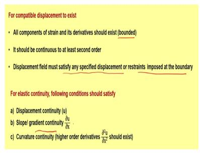
For compatible displacement to exist, now what is the whole idea? When some force act on a body whether it is under stress equilibrium, whether it is compatible, these are some of the questions we need to answer. So for compatible displacement to exist, all components of strain and its derivative should exist which means it should be bounded. It should be continuous to at least second order.
