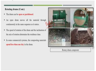
This is another unit of the rotary drum. So, a drum about 3.35 meter in diameter and 36.58 meter long as a daily capacity of approximately 50 tons with a residence period of see here residence period is 3 days this is what the major benefit. So, you see here the capacity is also 50 tons, now for 50 tons per day for windrow composting facility will be required huge amount of area for the degradation process and even degradation time also it goes to minimum 30 days and maximum goes to 90 days.
