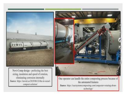
This is another reactor Novi-Comp design that is the best sizing, insulation and speed of the rotation eliminating corrosion internally. This is the blade is available in this reactor. So that the entire material will get mixed completely. So, feeding these reactors is the same reactor that you can see.
