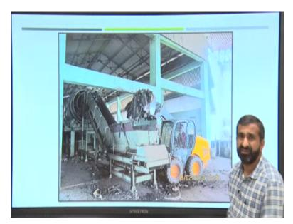
So, once this waste will dry for 30 days, it will feed into the trommel. Trommel is nothing but a filter. So, they are feeding that vehicle is feeding into the first trammel.
