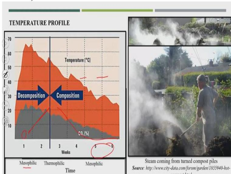
And now here finally, the temperature profile will be initially, decomposition and finally, it will be the completion of entire material. By that way we can understand.
