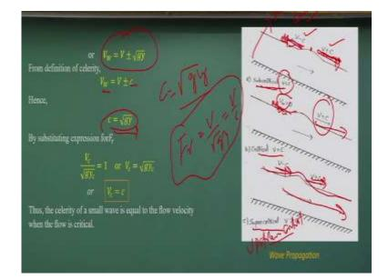
If I rearrange it, I will get  $V_w = V \pm \sqrt{gy}$  and c stands for the celerity that is what we are looking with the V value. So, the celerity comes out to,  $c = \sqrt{gy}$ . So, if you try to understand it that is what we are talking about. So when you have flow Froude numbers  $\frac{v}{\sqrt{gy}}$  or  $\frac{v}{c}$  you can understand it what it happens to the Froude numbers. It is a very simple thing what I try to show you.
