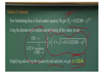
And then we are just substituting the relations. Similar way the upstream flow Froude numbers we can write in terms of the  $V_1$  velocities and we can have a relationship between  $y_2$  by  $y_1$  and that is what will give us a relationship with a flow Froude numbers that is what we are giving it and these equations because these are functions of z, but you can see it is not a linear equation, so you have to do hit and trials.
