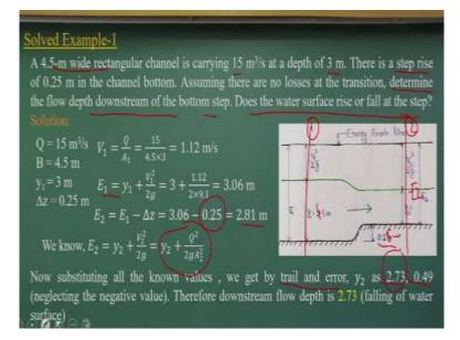
Let us have very simple problems to solve it. A 4.5 meters wide rectangular channel is carrying the discharge is 15 cumec at the depth of 3 m. There is a step rise 0.25 m and if that is the conditions determine the flow depth downstream of the bottom step. Does the water surface rise or fall over the step? So if you look at these problem, it is a very easy problem that there is a rise of the bed.
