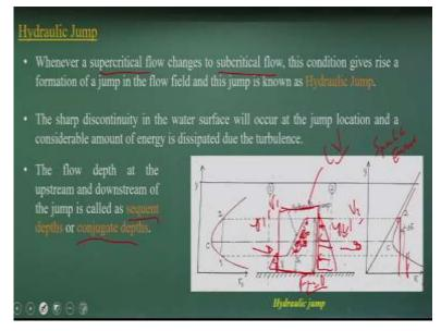
Already we have discussed specific energy, let us come back to the hydraulic jump. The hydraulic jumps it happens when a supercritical flow changes to the subcritical flow. That means very simple way but if you look at in terms of flow Froude numbers the supercritical flow where you have inertia forces is larger than the gravity force. When that changes happen as terms of force that is the mechanism happens from supercritical to subcritical.
