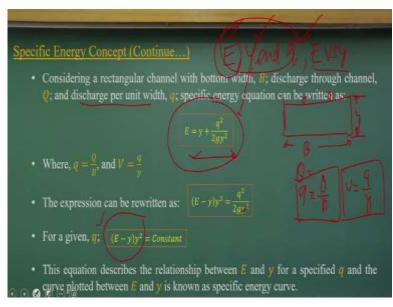
So considering that now if you look at these equations, it is a very simple way, many of the time we can consider the river as a rectangular channel, it has assumptions now. If I consider river is a simple rectangular channel, so having a B width and y is the depth of flow, I can consider channel is a rectangular channel, these are assumptions, it is also quite valid.
