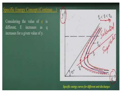
Let us understand the specific energy concept in a river point of view. Let me consider the river width variation are happening. The same discharge of q is coming it with variations there. Because of that as the width increases, the q will decrease, smaller q, the discharge per unit width will be decreasing. So if that is the conditions and that means if I have the conditions the discharge width is varying it from  $q_1$  to  $q_2$ .
