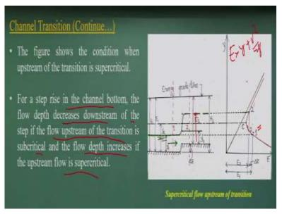
So looking that we can always make it like very interestingly these figures is indicating for us. So if I have this subcritical, the flow conditions will be, look these conditions that when the flow is supercritical at the upstream levels that is where the point one is here, in that case the solutions will be the 2A that is what two points the flow depth is going to increase okay. Flow depth is going to increase and you can find out.
