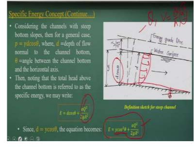
Now if you come into that river having bed slopes, it is not the flat. So in that case that means if the river is having this  $\Theta$  angle of the slope that is the real condition the river can have a very gentle slope or the mild slope like the Brahmaputra river the slope is in Assam valleys is about 1 by 10,000 or 1 by 8000 slope that is very gentle slope, but if you go to the Himalayans the slope could be an order of 1 by 20.
