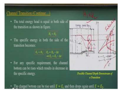
If you look at that as we have considered there is no energy losses, so energy gradient lines can be like this. So  $H_1 = H_2$ , but the specific energy at this  $E_2$  because energy gradient this flat is here so specific energy will be at the two locations will be  $E1 - \Delta z$ . So if the  $\Delta z$  is a rise, the specific energy drop will be there that is what will be the  $E2 = E - \Delta z$ , very simple thing because of increasing the level.
