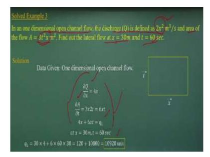
This is a very simple problem again. In a one-dimensional open channel flow that is when we are talking about only x directions, discharge  $Q = 2x^2 \text{ m}^3/\text{s}$ . So area is given as a function of t and x. Find out the lateral flow at x = 0 and t = 0. So basically, you want to find out the  $\frac{\partial Q}{\partial x}$  and  $\frac{\partial A}{\partial t}$  then you substitute to find out what will be the qL.
