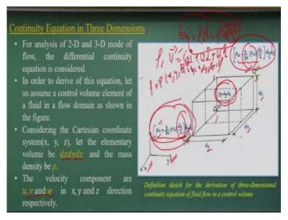
Let us start to derive the continuity equation in three dimensions. Before that, let me talk about that you have to consider control volume and basically when you try to derive the continued equation in three dimensions, our control volume is infinitely small, is very small control volume we consider and we also assume the velocity field, the depth variations, area variations.
