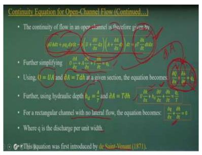
So, the influx part, the outflux part that's what the net change of the mass within this control volume which is the open channel control volume with lateral flow of  $q_L$  per unit length. So that way you can look at this equation which is just a mass conservation equation of influx, outflux and changing the mass within the control volume that is what if you simplified it, it comes like this.
