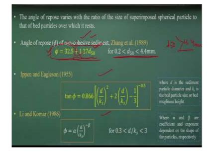
Many of the times we go for more details like for a non-cohesive soils like sand soil, we try to find out what could be the angle of repose with these empirical equations, which establish a relationship between angle of repose and the d50, d50 stands for diameter at the 50% finer. So, we can empirically establish it what could be the angle of repose if we just know the d50 value.
