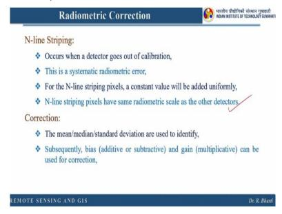
So it occurs when a detector goes out of calibration. So here this is the problem when you are having out of the calibration. So this is a systemic radiometric error, for N-line stripping pixel a constant value will be added uniformly again. N-line stripping pixel have same radiometric scale as the other detectors then correction is again the same.
