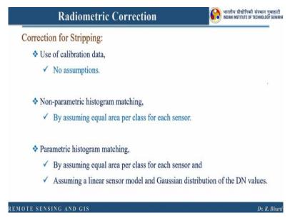
So here, when how do we correct? And what is the advantage and what is the assumption? So here you can see use of calibration data, calibration data of this sensor, then nonparametric histogram matching by assuming equal area per class for each sensor. The next is parametric histogram matching by assuming equal area per class for each sensor and assuming a linear sensor model and Gaussian distribution for the DN values.
