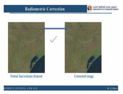
So here this is the example when you are having partial line or column dropout and this is the after correction. So this example I have put just for you to see the changes or to see the problem before correction and after correction. So you will better understand this particular error. Now next is N-line stripping.
