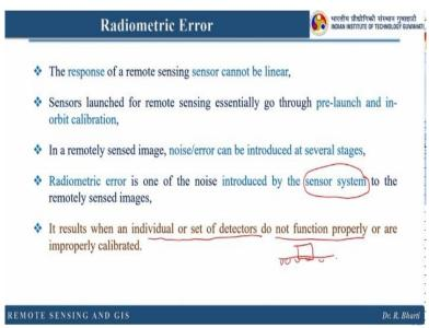
The response of a remote sensing sensor cannot be linear. So what does it mean? So it means when you plot this sensitivity of a detector, what happens? It will be like a gaussian distribution, so if you see there is a peak where it is sensitivity is maximum. But in other places, it is sensitivity is not up to the mark. So what happens? If we have to tell that what is the sensitivity of a detector then we use a term like FWHM. I hope you remember.
