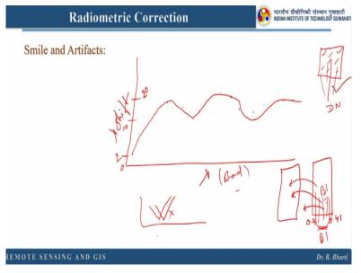
So if you see the corrected spectra and this is the wavelength shift, so this will be the wavelength shift and here you have wavelength or maybe let us call it band. So you will find there is 5, 10, 15 nanometer shift. This is not the measured spectra here we have plotted the shift spectra with respect to different bands. So if there is a change in some particular band, if there is a change of let us say this is maximum in this particular case.
