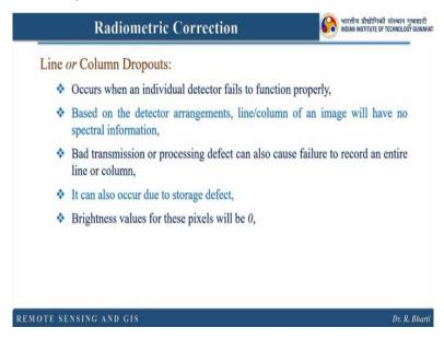
So what do you mean by line or column dropout? There we had some random pixels, random bad pixels. But here it will be like continuous. So it occurs when an individual detector fails to function properly. So here what is happening, you will not have any data for that particular detector. So that particular detector has failed to record the data and that is for the entire scene.
