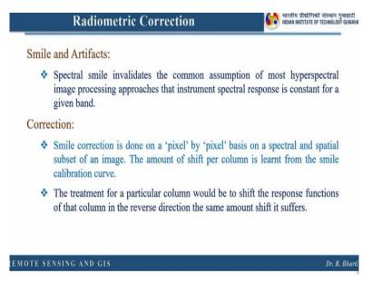
So spectral smile invalidates the common assumption of most hyperspectral image processing approaches that instrument spectral response is constant for a given band or a given material. So here you have understood this and the correction is a smile correction is done on a 'pixel' by 'pixel' basis on a spectral and spatial subset of an image. The amount of shift per column has learned from the Smile calibration curve.
