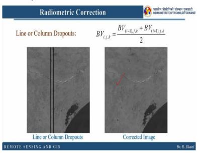
So here this is one example where you can see these 2 particular lines, they are basically line or column dropouts. So I made this line thicker, so that you can see this very easily but when you zoom it, it will be very thin line, why because one pixel just see, just imagine, if this is 1000 by 1000 pixels, so in that case one pixel, what will be the dimension of that pixel that will be lesser than this line. So you have to carefully go through the data before you are going to use it.
