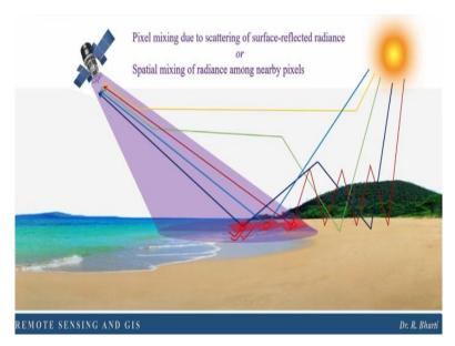
Now, next problem is adjacency correction. So adjacency effect is basically this is very critical. Now, you have to understand this particular case, in this particular case, what is happening sun is illuminating our surface and a sensor is active in this particular area and it is measuring the energies which is coming from different sources, so what is happening suppose if you have a pixel and they are lying next to each other.
