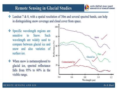
Landsat 7 & 8, with a resolution of 30 meter and several spectral bands, can help in distinguishing snow coverage and cloud cover from space. Specific wavelengths are sensitive to snow. Such wavelength are widely used to compare between glacial ice and snow and also varieties of surface ice. When snow is metamorphosed to glacial ice, spectral reflectance falls from 95% to 60% in the visible range.
