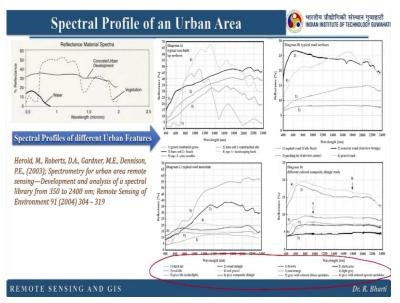
So, you can see here the vegetation, concrete and water body they are having different spectral profile right, and it can be used to identify different classes of urban right, here you can see different profiles associated with different objects. Right, and how they are different from each other, this is one of the potential areas where you can utilize the high spectral resolution information. So, this is in case of Urban Studies.
