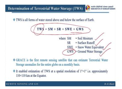
So here this is the equation. I hope you are familiar with this TWS is equal to SM plus SR plus SWE plus GWS where SM is soil moisture SR is basically surface runoff, SWE is basically your snow water equivalent GWS is basically your ground water storage. So basically we want to derive this one if we know all other parameters right. Grace is the first remote sensing satellite that can estimate terrestrial water storage anomalies for the entire globe on a monthly basis.
