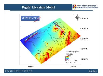
Now, let us see what exactly we mean by this digital elevation model and how it is going to help me now you are familiar that z value here corresponds to altitude, but in satellite remote sensing data, we have digital numbers it can be reflected or emitted or backscattered value, but here you are having altitude value height information. So, is there any way we can merge these 2 information together.
