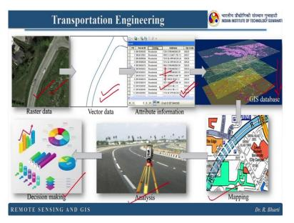
This slide gives you the overall understanding how this remotely sensed and GIS can help you in Transportation Engineering. So, here we have used this raster data and then we have converted into vector by digitizing or maybe you can use the automatic extraction techniques. Then these are the attributes which we have attached to this particular data by conducting a field investigation.
