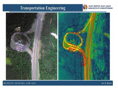
This is a very interesting work which has been done to identify the truck resting areas. So here you can easily find by using this thermal remote sensing data that some of the vehicles are of dark colour. These are the black one right. So that means these trucks are lying here for a long time rest are basically if you can see all these. So, here whichever is coming in the red there, this is a temperature data.
