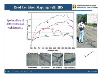
This already I have explained you in my previous lectures. Where this hyperspectral remote sensing data is used to identify the paving material and surface condition another example I showed you for the identification of road condition using the spectral profiles. In another work I explained you how this remote sensing or in particular hyperspectral remote sensing can be used for the aging and deterioration studies.
