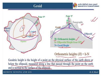
Let us assume this is the topography here. And here you have equator ellipsoid surface and this is the point for which I want to measure the height. So, that reference will be from Geoid because the sea surface level is our base level right. So, if you see the major and minor axis here, so, the major is A and minor axis is B. Now, here if you draw a line or perpendicular, you can see here this is your h which I expressed in a previous slide.
