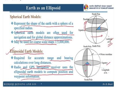
Let us see, when we consider our Earth as spheroid what happens and when we consider it as spheroid what happens. So, spherical Earth model represent this shape of the earth with sphere of a specified radius right, you might have seen this kind of figure many places. So, here basically this gives you the latitude and this is the parallel so, and this is equator. So, how it is moving.
