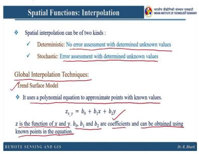
Spatial interpolation can be of two different types. So, first one is deterministic and second one is stochastic. So, in deterministic basically no error assessment with determined unknown values whereas, in stochastics error assessment with determined unknown values. So, this is the basic difference between the stochastic and deterministic and accordingly you have to choose which method you want to perform or apply for this spatial interpolation.
