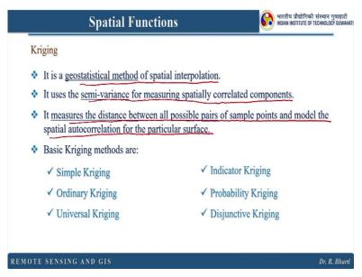
Now, the next method is kriging. It is a geostatistical method of spatial interpolation it uses a semi-variance for measuring spatially correlated components, it measures the distance between all possible pairs of sample points and model the spatial auto correlation for the particular surface. Basic kriging methods are simple kriging, ordinary kriging universal kriging and so on. You can search for this.
