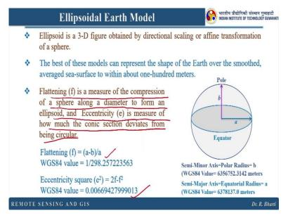
So, ellipsoid is a 3D figure obtained by directional scaling or affine tough a transformation of a sphere. The best of these models can represent the sphere of the earth over the smooth average sea surface to within about 100 meters. So, you can see this particular figure. So this is our earth and these are the pole and equator. And when we see semi minor axis and measure axis, so basically the major will have the greater value.
