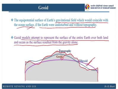
So, that is known as Geoid the Equipotential surface of Earth's gravitational field, which would coincide with the ocean surface if the earth were undisturbed and without topography. So, that will exactly match with your sea surface. Geoid model attempt to represent the surface of the entire Earth over both land and ocean as the surface resulted from the gravity alone.
