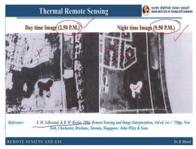
So let us see some example how this daytime and night-time images are coming up. So let us se this daytime which is at 2:50 p.m. right, and this is 9:50 p.m. So we assume that this time the temperature is maximum on the surface and this is night time when we expect that it has cooled down. So here you can see this is some kind of water body and it is having contrast.
