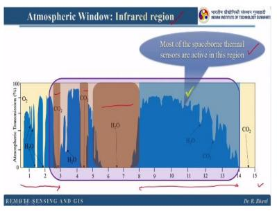
So I have another diagram, here you can see this is only for the infrared region, remember, this is for the complete infrared wavelength where we consider that till this 3 micrometre or 2.5 micrometre basically we have the reflected energy. So whatever energy sensed by our sensor that will be reflected from the surface, whereas 3 to 16 micrometre or here it is up to 15 micrometre, the energy which are emitted from the surface they are captured, right.
