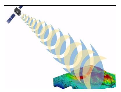
So this is one example, where I will demonstrate how we are using this active remote sensing and how we are illuminating the surface and how the pulses have been sent and received, right. So let us see here this is my microwave sensor which is illuminating this particular surface and the same time once it reaches to ground and it interact with the object then immediately it will back scatter.
