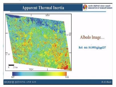
And this is the albedo image, so now you can see this is when we are using temperature data, So temperature data of ASTER is having 90 meter resolution, whereas albedo has been calculated using the 0.4 to 2.5 micrometre wavelength bands. So here your resolution is 30 metre. So this difference you can easily see here. So this is having good spatial resolution compared to your thermal data, right.
