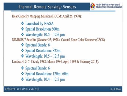
So first one is heat capacity mapping mission that was launched in 1978 right. Then Nimbus 7 satellite this was in 1978 again, then Landsat 4, 5, 7, 8, now we have Landsat 8, recently launched, which was launched in February 2013 and this is one of the very popular data which is used in thermal remote sensing. So it has many other bands, but the thermal bands are very useful.
