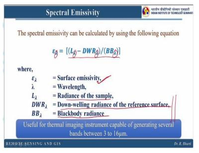
So the spectral emissivity can be calculated by using the following equation and here this is the variables. So here the surface emissivity can be calculated when you are having radiance of the sample, down-welling radiance of the reference surface and blackbody radiance. So when you are having all this information you can easily find out spectral emissivity, why spectral? Because everywhere we are using this lambda.
