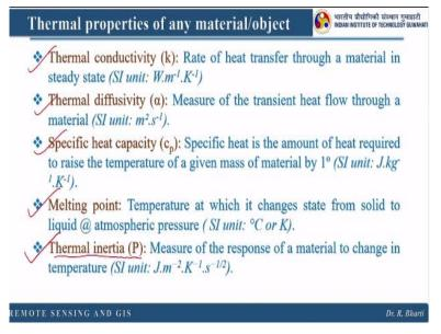
Now thermal properties of any material or object that are listed here. So first one is thermal conductivity, second one is thermal diffusivity, third one is specific heat capacity, fourth is melting point and thermal inertia. So I hope you are familiar with thermal conductivity, thermal diffusivity, specific heat capacity, melting point, but I guess this will be new to you, right.
