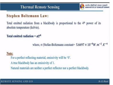
The total emitted radiation from a black body is proportional to the fourth power of it is absolute temperature. So total emitted radiation is equal to sigma T to the power 4, where sigma is the constant and T is the temperature, right. If you know temperature you can calculate the total emitted radiation. If you know total emitted radiation and sigma is known then you can calculate the temperature, right.
