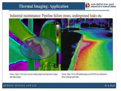
Now the next one is industrial maintenance. So here this is one example where pipeline failures zone right. Suppose you have a petroleum pipeline and you want to find out what are the vulnerable zones where it is likely to get failure or maybe leakage, right. So if you take thermal images then you can easily find out where it is supposed to be or it is likely to be failure, right.
