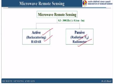
Here also we have 2 types of sensing. First one is active sensing and another one is passive sensing. So in active we call it backscattering RADAR, in passive it is radiation or radiometre can be used.
