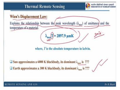
Now how do we find out the lambda max, where is the peak wavelength of emittance. So for that we have to refer this Wien's displacement law. Here it explains the relationship between the peak wavelength that is lambda max of emittance and the temperature of a material. So basically here if you see this equation, the lambda max is unknown. Suppose we do not know the lambda max of any material, right.
