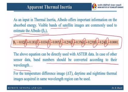
So in apparent thermal inertia as an input in thermal inertia albedo offers important information on the absorbed energy, visible bands of satellite images are commonly used to estimate the albedo, right and here in case of ASTER data you can straight away use this particular equation, right.
