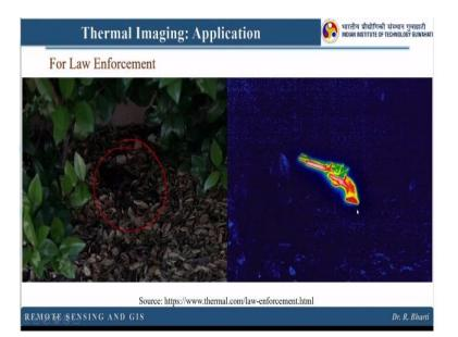
Now the next one is for law enforcement, here this gun was hidden, right, but here it is very evident like this is the gun lying in this particular location. So you can easily track which we cannot do or which was hidden or camouflaged in visible range, right. So there are few advantages which you cannot have with any other wavelength region.
