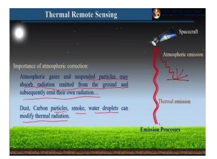
Now let us understand the importance of atmospheric correction in thermal remote sensing because here you have scattering and absorption and once you have absorption you will have emittance. So that is very clear from previous slides. Now what exactly happens here, the atmospheric gases and suspended particle may absorb radiation emitted from the ground and subsequently emit their own radiation.
