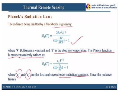
Then the next one is Planck's Radiation Law. So the radiance being emitted by a blackbody is given by this formula where K is Boltzmann constant and T is the absolute temperature. The Planck function is more conveniently written as this and where C1 and C2 are basically the first and second order radiation constants, right.
