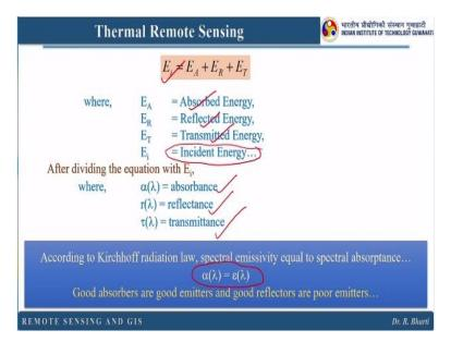
Now let us see this incident energy which is Ei = absorbed energy then + reflected energy + transmitted energy, right and when you divide by this incident energy what will happen? This will be absorbed, reflectance and transmittance, right. So according to Kirchhoff radiation law, spectral emissivity equal to spectral absorptance. So here this is clearly written. So good absorbers are good emitters and good reflectors are poor emitters.
