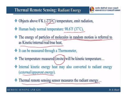
So that emits radiation. So any object above this particular temperature will emit radiation, right. Human body normal temperature is this one, so all the time we are emitting some energy, that we can see in the thermal imaging images, right. The energy of particles of molecules in random motion is referred to as kinetic, internal, real or true heat. So this is known as kinetic temperature right or sometimes internal temperature, real heat or true heat.
