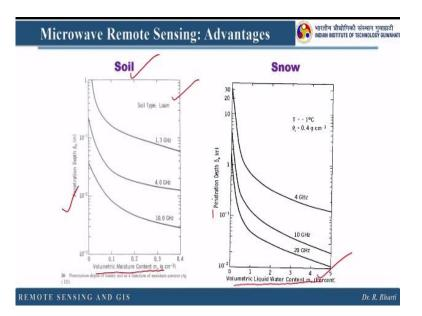
Here you can see the penetration depth for soil, this is the volumetric moisture content, so when you are having more moisture content your penetration will be less or more that you can see from here. In case of snow also as you are increasing the volumetric liquid water content then percentage depth will change, right.
