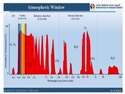
So these wavelengths, here you can see the red colours are basically showing the atmospheric transmittance, right. So here these wavelengths are allowed through our atmosphere to reach our surface and then it can travel back to the space. So there is no hindrance in our atmosphere for these wavelengths, but not all the wavelengths are completely free from this absorption and scattering.
