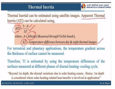
So how do we calculate this thermal inertia, so a very generic formula this is known as apparent thermal inertia, can be calculated using this satellite images where this is for initial assessment. Remember ATI that is basically apparent thermal inertia value is equal to 1 - albedo divided by delta T. Delta T is the temperature difference between day and night thermal images.
