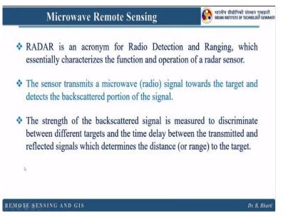
So what exactly RADAR means, RADAR is an acronym for radio detection and ranging which essentially characterize the function and operation of a RADAR sensor. The sensor transmits a microwave signal towards the target and detects the backscattered portion of the signal, the strength of the backscattered signal is measured to discriminate between different targets and the time delay between the transmitted and reflected signals which determines the distance to the target.
