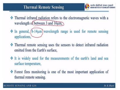
And the next point is, in general 8 to 14 micrometre wavelength range is used for remote sensing application, why so? Because in 8 to 14 micrometre you have good atmospheric transmission, do you remember that atmospheric window slide, my second slide of this lecture, there I have explained why this 8 to 14 micrometre wavelength range is preferred, because of the high atmosphere transmission.
