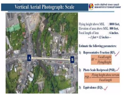
In this particular case I have kept this A and B here and they are separated with some distance and here we have flying height above MSL that is 8,000 feet. Elevation of area above MSL that is 800 feet, focal length of lens that is 6 inches and here you have to calculate RF, PSR and EQ and you just see the next slide after you have done with the calculation.
