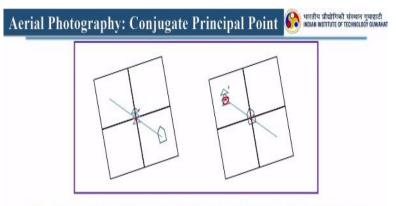
In a stereopair, identified Principal Point (PP) of a photograph can be located in the other one. This point is know as Conjugate Principal Point (CPP).
