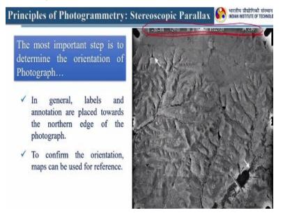
So now let us start with parallax. So what do we mean by stereoscopic parallax. So here the most important step is to determine the orientation of photograph. In general labels an annotations are placed towards the northern edge of the photograph. So if you see this is the northern edge of this photograph. To confirm the orientation map can be used for reference. You can use some previous images or the maps to reorient this if by mistake this has been wrongly put.
