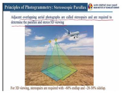
So here what exactly we are doing we are going to do the overlapped aerial photography. So adjacent overlapping aerial photographs are called stereopairs and are required to determine the parallax and 3D viewing. So here this is the ground and here for the first position I have capture this particular area. Now I have changed the position and then I have captured with some overlap and then we can have the stereopairs.
