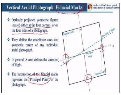
So when remote sensing started we started with the normal camera if you find old vertical aerial photographs you will find there are several marks printed on the photographs. This I am talking with respect to printed aerial photographs right and here we are talking about Fiducial mark. So optically projected geometric figures located either at the four corners or on the four sides of the photograph and they are known as Fiducial marks.
