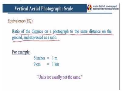
Now let us understand equivalence. So ratio of the distance on a photograph to the same distance on the ground and expressed as a ratio. So here basically ratio of the distance on a photograph to the same distance on the ground and expressed as a ratio right. So for example 6 inches=1 meter or 9 centimeter=1 kilometer and usually these units are not same in
