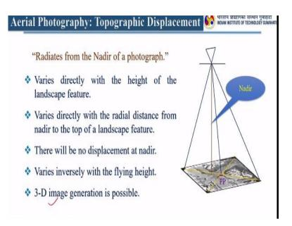
The topographic displacement they radiates from the Nadir of the photograph. So here we have Nadir varies directly with the height of the landscape features and varies directly with the radial distance from Nadir to the top of the landscape feature. There will be no displacement at Nadir because you are looking above that varies inversely with the flying height and when you have this you can always generate 3D images.
