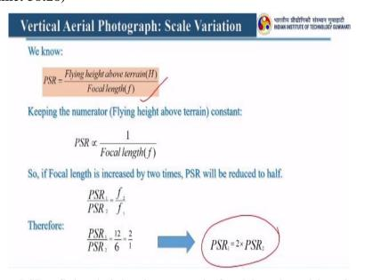
So here we know PSR= flying height above terrain/focal length and keeping the numerator flying height above terrain constant PSR is directly proportional to 1/focal length. So if focal length is increased by 2 times PSR will be reduced to half. So therefore there will be change in the PSR with this right.
