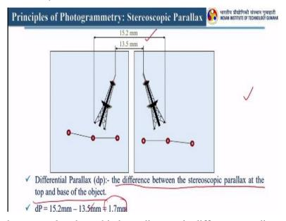
Here this is another example where this base distance is different, top distance is difference because in both the images none of them were vertical photographs right. When you have such images with you, you can always calculate the distance between these two right and you can always calculate the distance between bottom and differential parallax you can calculate using the difference between the stereoscopic parallax at the top and base of the object.
