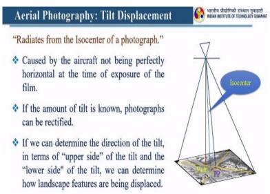
Then the displacement is the shift in the position of the landscape features that does not alter the perspective characteristic image. So here again curvature of the earth is negligible, tilt and topographic relief. So tilt displacement it radiates from the Isocenter of a photograph so here this is the Isocenter it is caused by the aircraft not being perfectly horizontal at the time of exposure of the film right.
