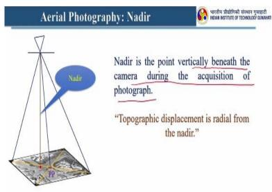
So Nadir is the point vertically beneath the camera during the acquisition of photographs right and here if you see this is the Nadir point so they are definitely different from each other right and topographic displacement is radial from the Nadir. So topographic displacement will be very less at Nadir as you go away of Nadir you will find more topographic displacement.
