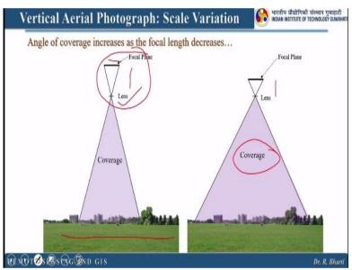
So this is one example I have put to understand what is the effect of focal length on the acquired image. So if you see here we have this is the focal plane, this is the lens and this is the area which we want to capture. So here you can see this is different and this is different. So if you see the coverage of this particular setup or this particular instrument is basically less.
