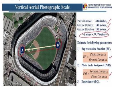
So for a vertical photograph I have taken this A and B location and their distance right. So you can easily measure the distance between these two points on the photograph based on the spatial resolution and assuming we have the ground distance we have visited that particular place and you have calculated the distance between these two or you have measured that. So here we have few known like what is the photo distance, what is the ground distance then ground elevation.
