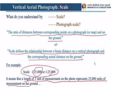
So let us start by what do you understand by scale and that too photograph scale because now we are talking about the photograph. So here this is the ratio of distances between corresponding point on photograph which is basically map and on the ground right so this is the ratio and in other words scales defines the relationship between a linear distances on a vertical photograph and the corresponding actual distance on the ground right.
