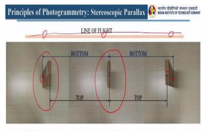
Note the displacement between the top and base of the storage towers in this photo stereopair.
