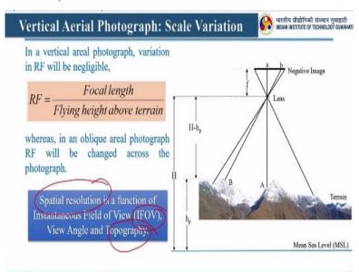
So apart from this scale there is very important to understand this variation because scale we identify for a particular object or for a particular scene but on ground we have this elevation different. So do this scale is consistent throughout the scene or they can vary place to place so that you need to understand. So in a vertical aerial photograph variation in RF will be negligible right because in vertical aerial photograph we assume distortion is very less and we are seeing from the top.
