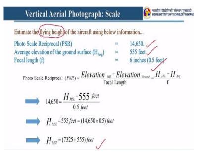
This is another problem where you have to estimate the flying height of the aircraft using following information. So here you have photo scale reciprocal average elevation of the ground surface and then focal length right. So how do you calculate the flying height now this is the reverse problem. Now you can always use the same equation by changing it and then you can calculate what is the flying height of your craft.
