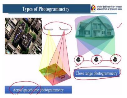
Now there are different types of Photogrammetry so first one is aerial photogrammetry or spaceborne photogrammetry and the next one is your close range photogrammetry. So here you can see different acquisition mode for this different types of Photogrammetry. So let us start with the first one. Here in case of aerial and spaceborne photogrammetry basically we rely on the sensors which are placed in space or in a aircraft right.
