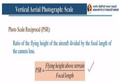
Similarly, PSR can be calculated using this focal length and flying height using this formula right.
