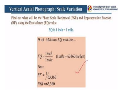
Now the next question is find out what will be the photo scale reciprocal and representative fraction that is RF using the equivalence value right an equivalence is 1 inch= 1 mile. So here this is the solution you can go through it, you can calculate it because this is very simple you just have to correlate your basic understand with the problem. So you have seen the different scale.
