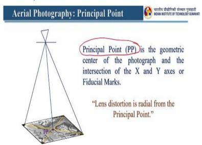
So in image basically it will look like this right so principal point is the geometric center of the photograph and the intersection of X Y axes or fiducial marks. So it is very important that you should able to identify principal point PP in your photograph. Lens distortion is radial from the principal point. So lens distortion will be minimum at principal point. So as you go
