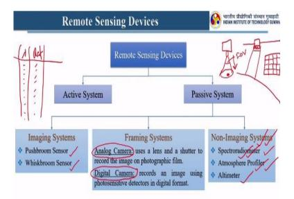
So let us understand what are the different types of devices available in remote sensing. So if you see here we have two different categories. First one is active system and next one is passive system. So I hope you remember this two terms. Active system means you have your own source of light when you are engaged in imaging. In case of passive system, we are using solar energy as source and here if you subdivide this passive system.
