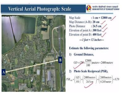
Here this is another example where AB are separated with this line and here you have map scale, map distance, photo distance, elevation of point A that is 300 feet and elevation of point B that is 400 feet. Now how do you calculate ground distance, photo scale reciprocal that is PSR right so you can calculate using this and PSR you can calculate using this.
