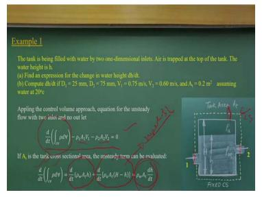
If it is that, apply the Reynolds transport theorems, okay? You apply the Reynolds transport theorems. You have the inflow and the outflow. There is no outflow in this case. In both the
