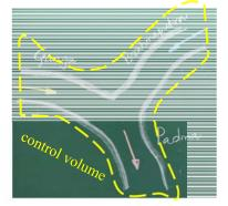
Appling the control volume approach, equation for the unsteady flow with two inlet and one out let
