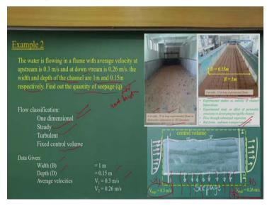
The water is flowing in a flume with a downward seepage average velocity at upstream is 0.3 m/s and at down stream is 0.26 m/s. the width and depth of the channel are 1m and 0.15m respectively. Find out the quantity of seepage (q).
