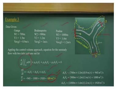
So, if I have width and the depth and velocity like this, so we can apply this continuity equations for this control volume, okay? For Ganga, Brahmaputra, Padma systems I have control volumes and all, I can have positive and the negative, okay?
