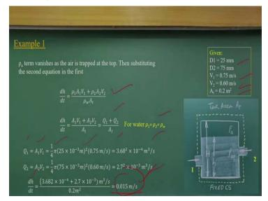
$\rho_a$  term vanishes as the air is trapped at the top. Then substituting the second equation in the first
