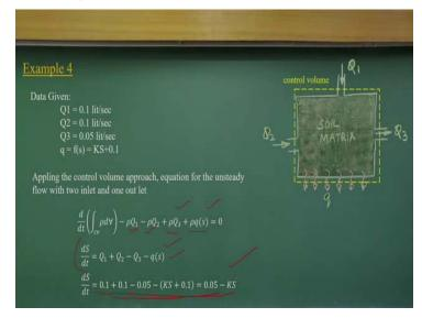
Now, if I substitute this equation, if you look at these inflows are the negative, outflows are positive, and Qx is the function of this. So, Appling the control volume approach, equation for the unsteady flow with two inlet and one out let
