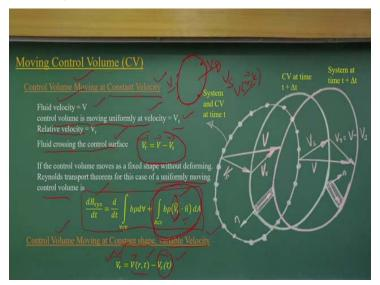
Now coming to a very interesting (()) (13:15) if I consider moving control volume like a ship which is moving with a velocity V. So, then, the concept will be the same. Only here we will talk about the relative velocity component. That means there will be fluid velocity V and control volume is moving with a velocity, let it be  $V_s$ . So, we need to know it, what will be the relative velocity  $V_r$  crossing through this control surface.
