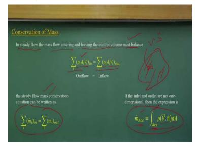
That is what again I am going to repeat it to tell you that further steady flow, mass flow entering the leveling control must be balanced. It is too packed, there is nothing else. Any system, if it is steady, it does not change with time, with respect to time. That means, what it indicates is that there is no change in the storage, mass flow, there is no change in the mass storage within this control volume. So, inflow should be equal to the outflow.
